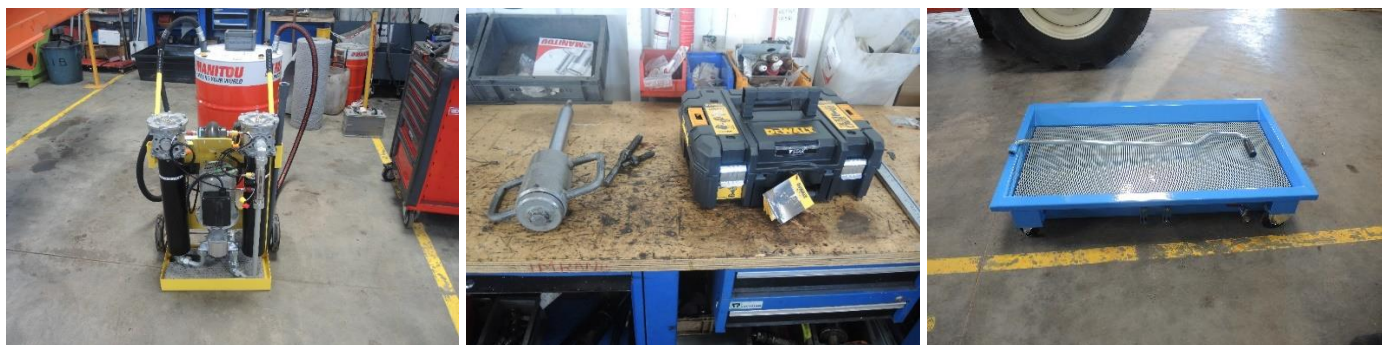
Figure 61 – Photos of the tools recommended and acquired to smooth the dismantling process
