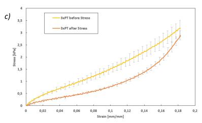
Figure 5.16: Study  $n^{\circ}1$  on enzymatic stress. Tensile tests on 3 explants, before and after introduction of collagenases and elastases (speed = 10 mm.min<sup>-1</sup>). Stress versus strain graphs. a) Before stress. b) After stress. c) Comparison of average curves.
