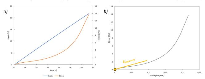
Figure 2.31: Tensile test on a skin explant. a) Raw curves: stress and strain as a function of time. b) Stress versus strain graph. Parameters: strain = 22% - speed = 1mm.min<sup>-1</sup>.
