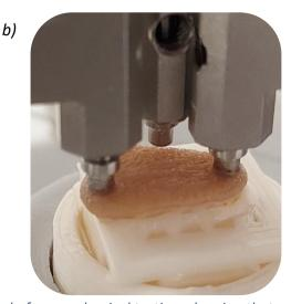
Figure 3.11: Photographs of a skin explant in the device before mechanical testing, showing that pre-tension can be applied to the explant. a) No initial pre-tension. b) Initial pre-tension (30% extension).
