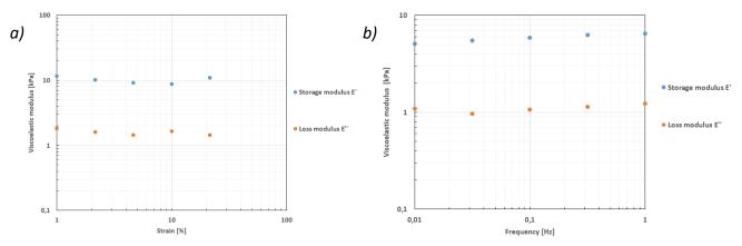
Figure 2.28: Dynamic tests on a skin explant. a) Strain sweep test (frequency = 0.1 Hz). b) Frequency sweep test (strain = 10%)
