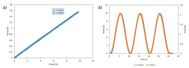
Figure 2.18: Results of mechanical tests with elastics. a) Simple traction (speed = 1 mm.min-1). b) Dynamic tests (f = 0.1 Hz - strain = 10%).
