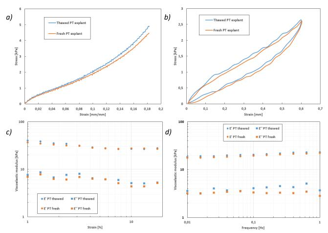
Figure 5.13: Freezing study: complete characterisation of the PT explant before and after a freezing period.
