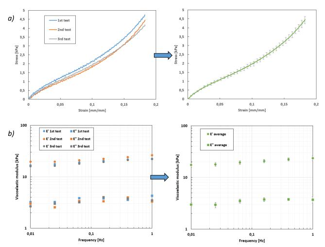
Figure 3.4: Reproducibility of tests on human skin explants. a) Reproducibility in tensile test (speed =  $10 \text{ mm.min}^{-1}$ ): 3 tests + average curve with standard deviation. b) Example of reproducibility of a dynamic test (frequency sweep at 10%): 3 tests + average curve with standard deviation.
