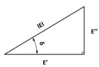
Figure 2.29: Relationship between the storage modulus E', the loss modulus E'', the phase angle  $\delta$  and the magnitude |E| of the complex modulus  $E^*$ .
