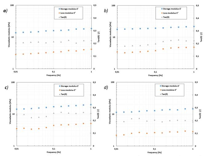
Figure 4.9: Results of frequency sweep tests on 4 human skin explants (strain = 10% -  $T = T_{amb}$ ). Graphs of viscoelastic moduli, and loss factor, as a function of frequency. Explants PD (a), PJ (b), PM (c) and PN (d).
