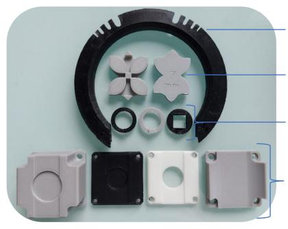
Figure 2.12: Photo of different 3D printed parts to adapt to different types of human skin samples.
