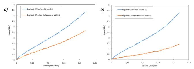
Figure 5.25: Study on collagenases, elastases, and inhibitors. Tensile tests on 2 different explants of the PI plasty: (a) CA explant before and after exposure to collagenases, and (b) EA explant before and after exposure to elastases. Stress versus strain graphs (speed = 10 mm.min<sup>-1</sup>).
