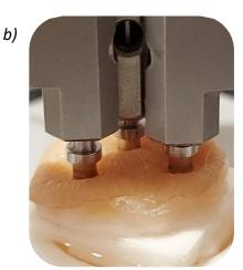
Figure 3.7: Photographs of the instrument's studs glued to the skin surface, showing different normal forces applied to the same skin explant: 3 mN (a) and 23 mN (b). The difference between the 2 pressures applied to the skin is clearly visible.
