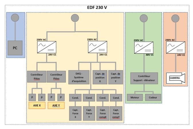
Figure A10: Single-line diagram of the power supply principle for our device.
