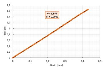
Figure 2.16: Tensile test results with a spring. Measurement of the spring stiffness constant:  $k = [3.85 \pm 0.05]$ N.mm<sup>-1</sup>.
