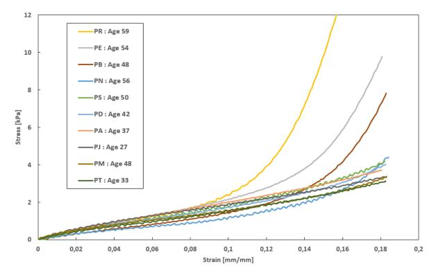
Figure 4.19: Results of tensile tests on all human skin explants (speed =  $10 \text{ mm.min}^{-1}$ ). Stress versus strain graph.
