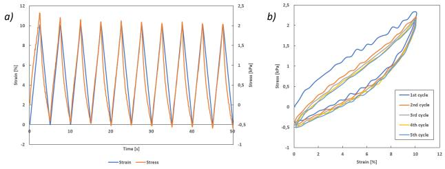
Figure 3.2: Preconditioning experiment on a human skin explant showing the Mullins effect, carried out using our instrumentation. a) 10 loading-unloading cycles. b) Superimposed stress-strain curves showing stabilisation of the mechanical properties of the skin from the 3rd/4th cycle.
