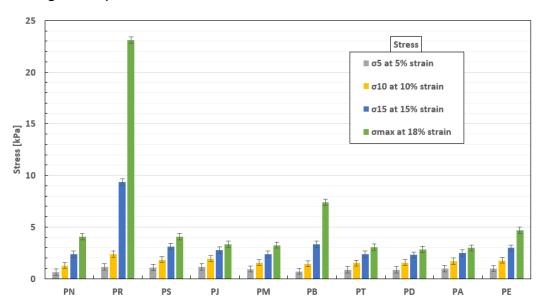
Figure 4.4: Results of mechanical tensile tests on human skin explants. Stresses measured for each explant, at different percentages of deformation (with force sensor measurement uncertainties).
