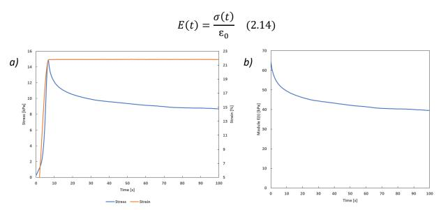
Figure 2.32: Stress relaxation test on a skin explant. a) Stress and strain as a function of time (raw curve). b)
