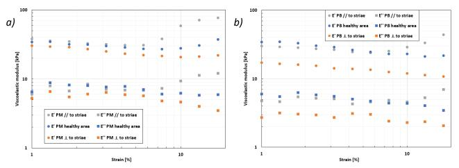
Figure 5.6: Study on stretch marks: strain sweep tests on 2 explants with stretch marks, in 3 load directions (f = 0.5 Hz). Graphs of viscoelastic moduli as a function of strain. Explants PM (a) and PB (b).
