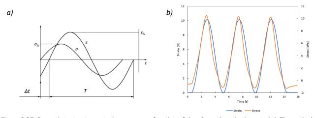
Figure 2.27: Dynamic tests: stress-strain curves as a function of time for a viscoelastic material. Theoretical curve (a) and experimental curve on human skin (b).
