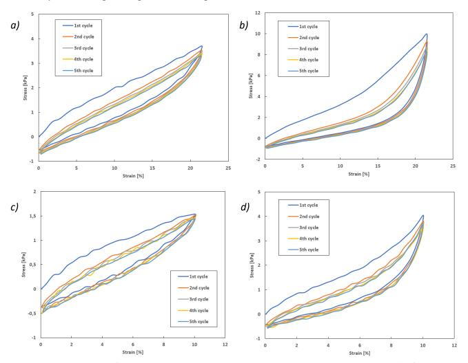
Figure 4.12: Results of cyclic mechanical loading-unloading tests on 4 human skin explants (def = 10% or 22% / speed = 10 mm.min<sup>-1</sup>). Stress versus strain graphs. Explants PA (a), PE (b), PT (c) and PR (d).
