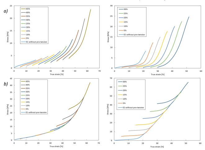
Figure 3.14: Tensile tests on 2 explants of human skin (speed = 10 mm.min<sup>-1</sup>) with different initial pretensions. a) Graphs with initial deformations respected. b) Graphs with adjusted stresses.
