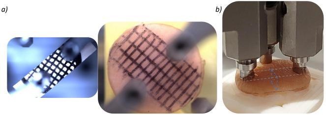
Figure 2.26: a) Analysis of the surface of the sample under stress using the camera and an ink grid (elastic band and pigskin). b) Section stressed in tension (human skin).
