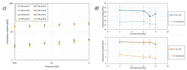
Figure 4.17: Study on the survival of a skin explant over time: PD explant, tested at D+2, D+6, D+7 and D+8.
