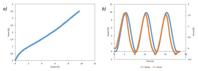
Figure 2.20: Results of mechanical tests on a sample of pigskin. a) Simple traction (speed = 1 mm.min<sup>-1</sup>). b) Dynamic tests (f = 0.1 Hz - strain = 10%).
