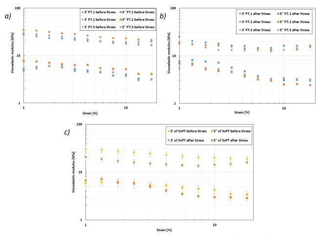
Figure 5.17: Study n°1 on enzymatic stress. Strain sweep tests on 3 explants, before and after introduction of collagenases and elastases (f = 0.5 Hz). Graphs of viscoelastic moduli as a function of strain. a) Before stress. b) After stress. c) Comparison of average curves.
