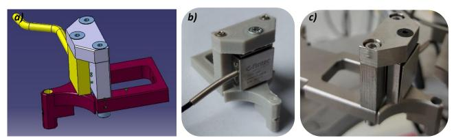
Figure 2.9: Prototyping of new arms with a vertical force sensor. a) Part designed in CATIA. b) 3D printed part. c) Machined part.
