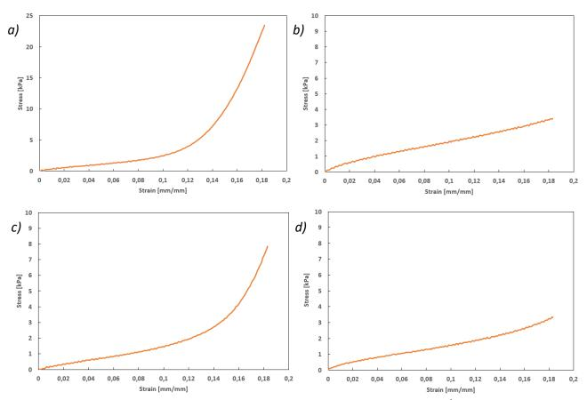
Figure 4.2: Stress - Strain curves for 4 human skin explants (speed =  $10 \text{ mm.min}^{-1}$ ). Stress versus strain graphs. Explants PR (a), PJ (b), PB (c) and PM (d).
