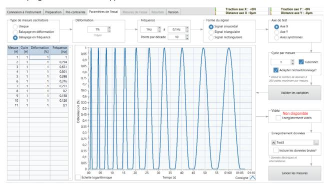
Figure 2.11: Example of a page from the software interface used to set up a mechanical test.
