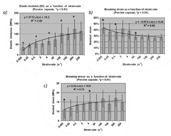
Figure 1.29: Effect of strain rate (0.005 to 250 s<sup>-1</sup>) on the mechanical properties of a porcine kidney capsule. a) Effect on  $E_2$  modulus of elasticity (last tensile phase). b) Effect on strain at break. c) Effect on stress at break – [Snedeker et al., 2005]
