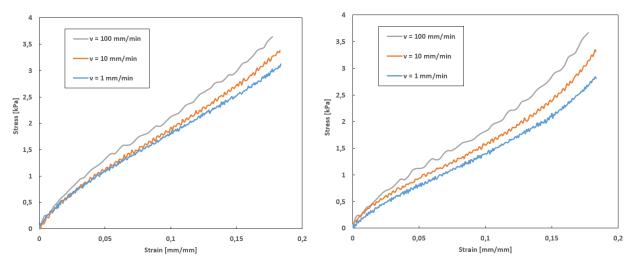
Figure 3.6: Influence of strain rate on the mechanical elongation behaviour of the explant. Tensile tests on 2 human skin explants (right and left graphics - speed = 1, 10 and 100 mm.min<sup>-1</sup>).
