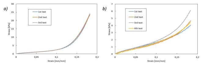
Figure 3.5: Other examples of the reproducibility of tensile tests on two human skin explants (speed =  $10 \text{ mm.min}^{-1}$ ). a) Experiment with very good reproducibility. b) Experiment with poorer reproducibility: error in the positioning of the skin for test no. 3, which does not follow the general trend in mechanical properties.
