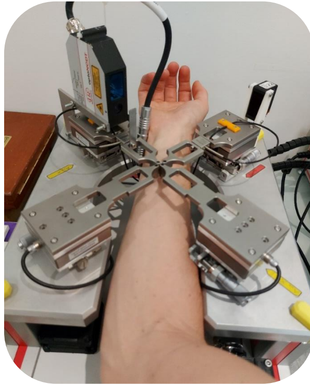
Figure C.1: Photo of the configuration of the device in "in vivo" mode with the forearm of a volunteer patient.
