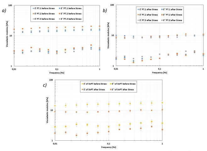
Figure 5.18: Study n°1 on enzymatic stress. Frequency sweep tests on 3 explants, before and after introduction of collagenases and elastases (strain = 10%). Graphs of viscoelastic moduli as a function of frequency. a) Before stress. b) After stress. c) Comparison of average curves.
