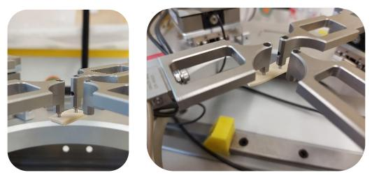
Figure 2.17: Mechanical test on an elastic band.
