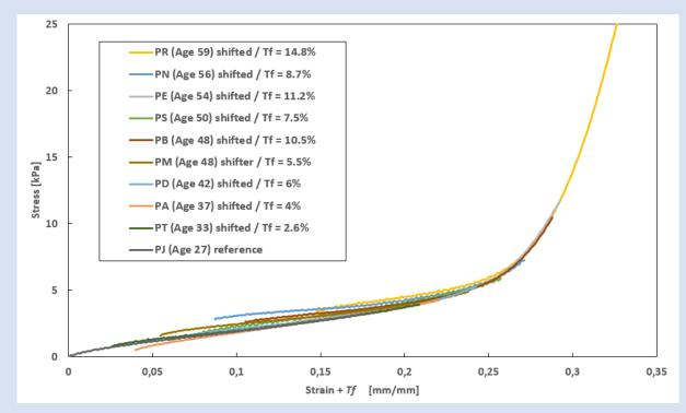
Figure 4.20: Translation of stress-strain curves of skins of different ages in order to establish a master curve (Tf = translation factor). Horizontal and vertical translation of curves having different mechanical behaviour.
