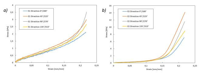
Figure 3.18: Mechanical anisotropy of human skin. Tensile tests on 2 human skin explants (speed =  $10 \text{ mm.min}^{-1}$ ) in different directions.
