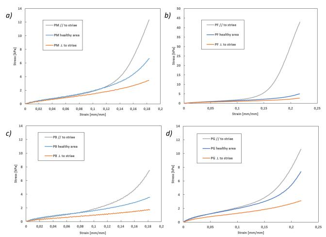
Figure 5.5: Study on stretch marks: tensile tests on 4 explants with stretch marks, in 3 directions of load  $(speed = 10 \text{ mm.min}^{-1})$ . Stress versus strain graphs. Explants PM (a), PF (b), PB (c) and PG (d).
