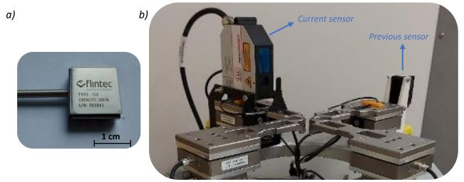
Figure 2.8: Measurement improvement. a) Photo of a miniature S-type force sensor used in our device. b)
