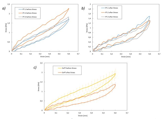
Figure 5.19: Study n°1 on enzymatic stress.  $5^{th}$  cycle of cyclic loading-unloading tests on 3 explants, before and after introduction of collagenases and elastases (strain = 10% / speed = 10 mm.min<sup>-1</sup>). Stress versus strain graphs. a) Before stress. b) After stress. c) Comparison of average curves.
