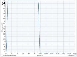
Figure 2.25: Static mechanical tests. a) Simple traction: linear ramp of imposed strain (Parameters: strain = 10% - speed = 6 mm.min<sup>-1</sup>). b) Stress relaxation: strain kept constant (Parameters: strain = 10% - time = 60s).
