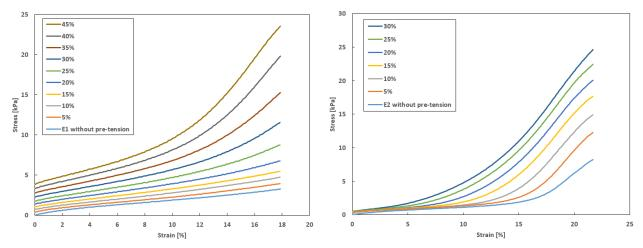
Figure 3.12: Influence of explant pre-tension on its mechanical behaviour in elongation. Tensile tests on 2 human skin explants (right and left graphics - speed =  $10 \text{ mm.min}^{-1}$ ) with different initial pre-tensions.
