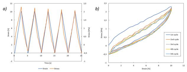
Figure 2.30: Dynamic load-unload test on a skin explant: stress-strain curves as a function of time (a) and as a function of the measured cycle (b). Parameters: strain = 10% - f = 0.2 Hz.
