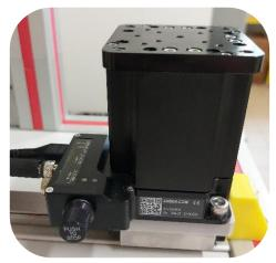
Figure 2.10: Specific support with integrated motor controllers and encoders.
