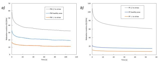
Figure 5.9: Study on stretch marks: stress relaxation tests on 2 explants with stretch marks, in 3 load directions (Parameters: tension = approx. 1 or 2 min / strain = 18%). Graphs of relaxation modulus E(t) as a function of time. Explants PM (a) and PF (b).
