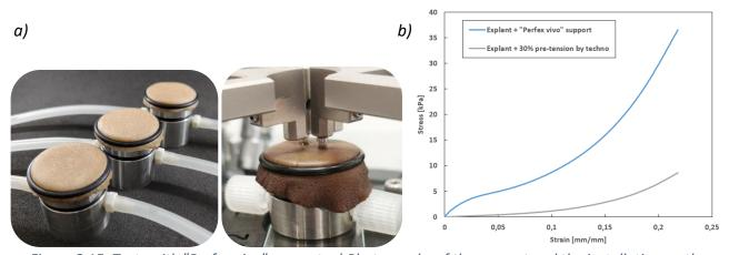
Figure 3.15: Tests with "Perfex vivo" support. a) Photographs of the support and the installation on the device. b) Comparison of a simple tensile test, on the same explant of human skin (speed=10mm.min<sup>-1</sup>), with the "Perfex vivo" support and with a pre-tension generated by the equipment.
