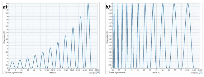
Figure 2.23: Dynamic mechanical tests: imposed strain sinusoids. a) Strain sweep (Parameters: strain = 1 to 10% - frequency = 0.1 Hz). b) Frequency sweep (Parameters: f = 1 to 0.1 Hz - strain = 1%).
