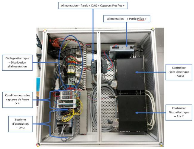
Figure A2: Photo of the "instrumentation box"
