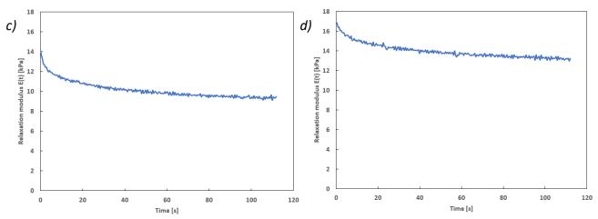
Figure 4.14: Results of mechanical stress relaxation tests on 4 human skin explants (Parameters: tension = approx. 2 min / strain = 18%). Graphs of relaxation modulus  $\frac{\sigma(t)}{\epsilon_0}$  as a function of time. Explants PA (a), PE (b), PM (c) and PJ (d).
