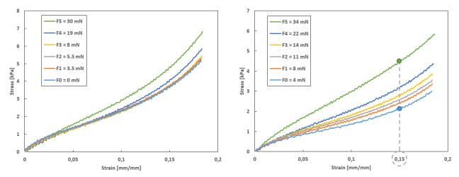
Figure 3.10: Tensile tests on 2 human skin explants (right and left graphics - speed =  $10 \text{ mm.min}^{-1}$ ) with different normal forces.
