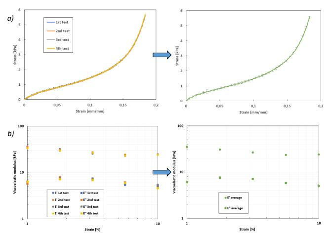
Figure 3.3: Repeatability of tests on a human skin explant. a) Tensile test (speed = 10 mm.min<sup>-1</sup>): 4 tests + average curve with standard deviation. b) Dynamic test (strain sweep at 0.5 Hz): 4 tests + average curve with standard deviation.
