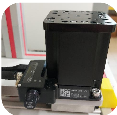
Figure 2.10: Specific support with integrated motor controllers and encoders.
