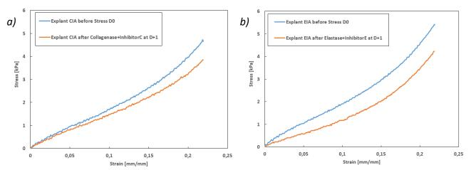
Figure 5.27: Study on collagenases, elastases, and inhibitors. Tensile tests on 2 different explants of the PI plasty: (a) CIA explant before and after exposure to collagenases + collagenase inhibitors, and (b) EIA explant before and after exposure to elastases + elastase inhibitors. Stress versus strain graphs (speed = 10 mm.min<sup>-1</sup>).
