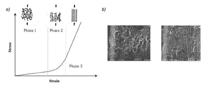
Figure 1.24: Non-linear behaviour of skin in tension. a) Typical stress-strain curve for skin and diagram of collagen fibres orientation – [Wilkes et al., 1973]. b) Scanning Electron Microscopy observation of rat skin collagen fibres: i) initial and ii) stretched state in tension – [Belkoff et al., 1991]
