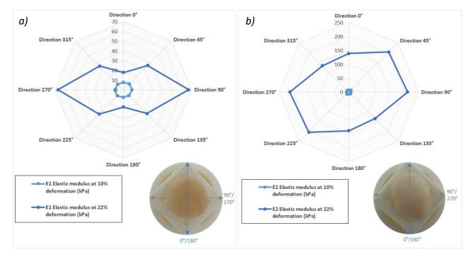
Figure 3.19: Mechanical anisotropy of human skin. Radar graph of the elastic moduli of the 2 explants.
