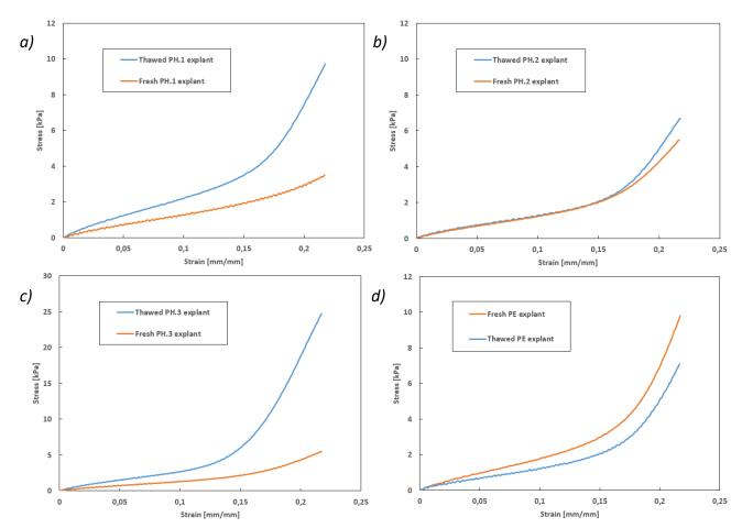
Figure 5.12: Freezing study: traction tests on 4 explants, before and after a period of freezing (speed =  $10 \text{ mm.min}^{-1}$ ). Stress versus strain graphs. 3 explants PH (a,b,c) and 1 explant PE (d).
