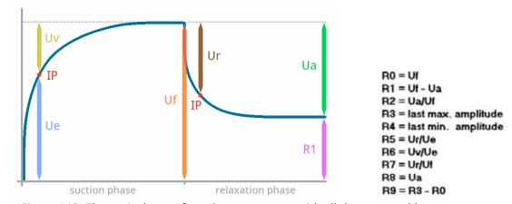
Figure A13: Theoretical curve for a Cutometer test, with all the measurable parameters.
