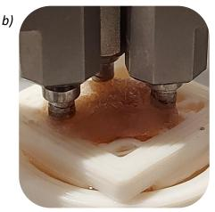
Figure 5.15: Study on enzymatic stress: photos of the PD explant in test configuration, before stress (a) and after 2 days of enzymatic stress (b). Visual observation of the explant clearly shows the degradation of the dermis caused by collagenases and elastases.
