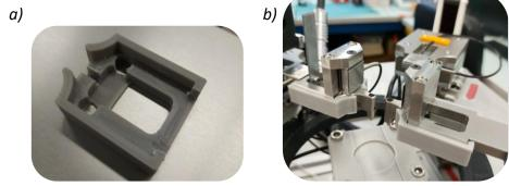
Figure A3: a) Photos of the 3D printed "arm mould" part. b) Photo of this part attached to the arms of the device.
