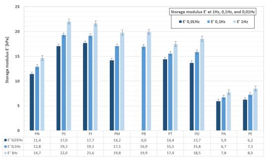
Figure 4.10: Results of frequency sweep tests on human skin explants. Storage modulus E' determined for each explant, at different frequencies (Notes: without the PR test (not carried out) and with force sensor measurement uncertainties).
