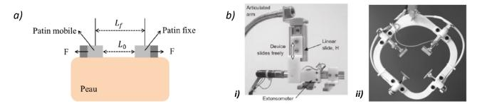
Figure 1.33: Extension tests. a) Schematic diagram of the test principle ( $L_0$  = initial pad spacing,  $L_f$  = final spacing) – [Azzez, 2019]. b) Extensometers used in vivo: i) uni-axial extensometer – [Lim et al., 2008]. ii) biaxial extensometer – [Capek et al., 2010]
