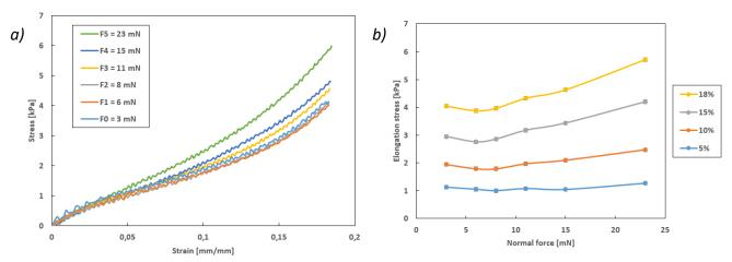
Figure 3.8: Influence of the compression force of the studs on the mechanical behaviour of the skin in elongation. a) Tensile tests on an explant of human skin (speed = 10 mm.min<sup>-1</sup>) with different normal forces. b) Elongation stresses measured, for a given deformation, as a function of the normal force imposed.
