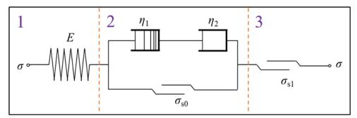
Fig. 6.1 Creep-fatigue rheological model.
