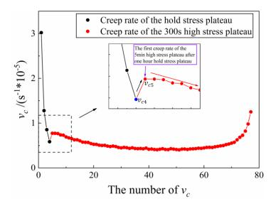
Fig. 3.7 Creep rate  $(v_c)$  for TCF test at 3 MPa confining pressure. The black dot is the  $v_c$  at the one-hour high-stress plateau, and the red dot is the  $v_c$  at the high-stress plateau during the fatigue creep stage.
