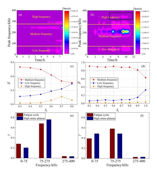
**Fig. 4.11** Probability density distribution of peak frequencies and ratio for the three frequency bands for every  $S_{l \, levels}$  in the USCF test (a and c) and TSCF test (b and d) (note: 0.3  $S_{l \, is}$  the T-stage). Fatigue cycle and high-stress plateau in different frequency bands as a percentage of AE frequency in the USCF test at 0.5  $S_{l}$  (e) and 0.8  $S_{l}$  (f).
