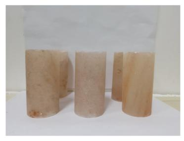
Fig. 2.3 Salt rock specimens.
