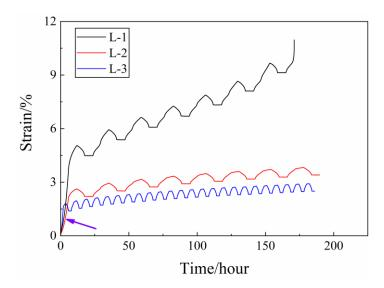
Fig. 5.3 Strain-time curves for three long-time creep-fatigue tests.
