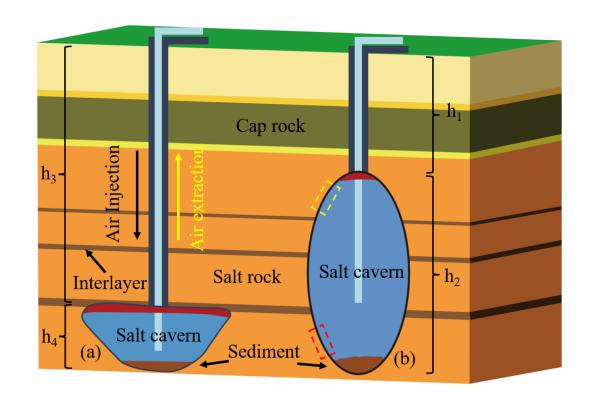
Fig. 3.15 Schematic diagram of two salt cavity shapes: horizontal dissolution cavity ( $h_1$  and  $h_2$  are the depth and height, respectively) (a) and vertical dissolution cavity ( $h_3$  and  $h_4$  are the depth and height, respectively) (b).
