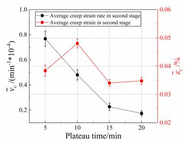
Fig. 2.11. Average creep rate and strain during the stabilization deformation (the second stage, II) under different plateau times.
