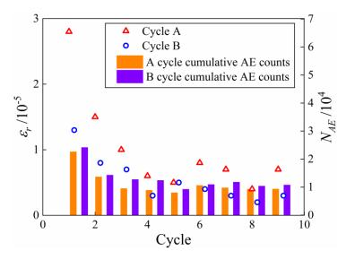
Fig. 4.16 Residual strain and AE counts statistics per cycle in 0.5 S<sub>l</sub> from USCF test
