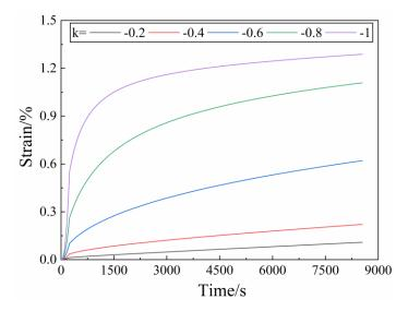
**Fig.6.14** Creep-fatigue curves under pure creep for different *k* values.
