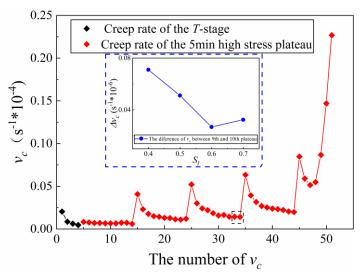
Fig. 4.6 Creep rate during USCF test
