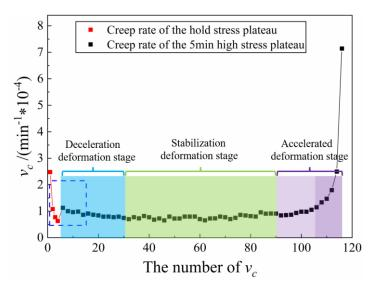
Fig. 2.10 Creep rate during the 5 min plateau time CCFT.
