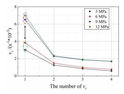
Fig. 3.8 The trends of the first four  $v_c$  values during the T stage under different confining pressure.
