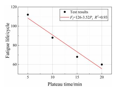
Fig. 2.14. Fatigue life for different plateau times.
