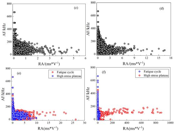
**Fig. 4.13** AF versus RA distribution during the USCF test (a) and TSCF test (b) at 0.5  $S_l$  (c) and 0.7  $S_l$  (d) in the USCF test and 0.7  $S_l$  (e) in the TSCF test. The fatigue cycle and high-stress plateau at 0.7 (e) and 1.0  $S_l$  (f) in the TSCF test
