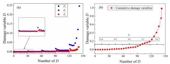
Fig. 4.14 Fatigue cycle and high-stress plateau damage variable development (a) and cumulative damage variable (b) in the USCF test. Damage includes the initial one-hour high-stress plateau  $(D_I)$ , fatigue cycles  $(D_f)$  and high-stress plateau  $(D_c)$ .
