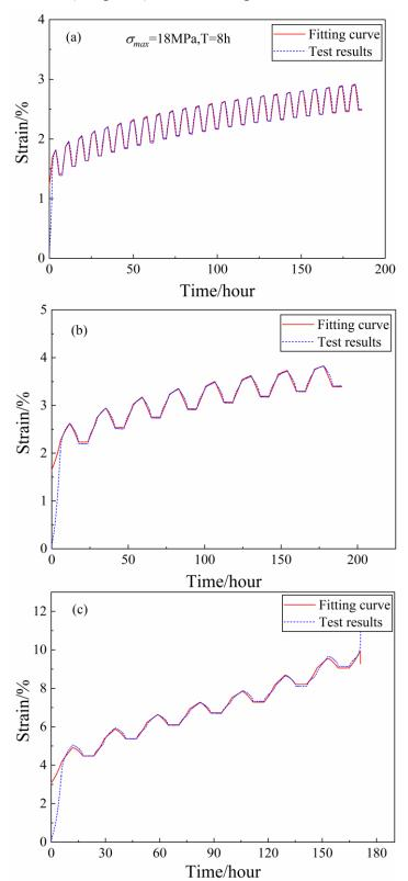
**Fig. 6.13** Comparison graphs of test results and fitting results, (a) long-term creep-fatigue test with a stress upper limit of 18MPa and a cycle duration of 8 hours, (b) long-term creep-
