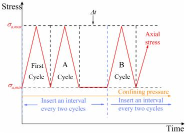
Fig. 6.10 Low stress interval fatigue test loading path.
