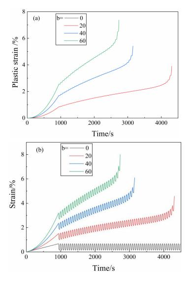
**Fig.6.24** Model deformation curves corresponding to different values of *b* (a) plastic strain and (b) total strain
