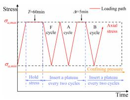
Fig. 3.1 Loading paths during the triaxial creep-fatigue (TCF) tests.
