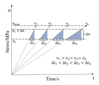
Fig.5.11 Schematic diagram of loading path
