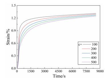
Fig.6.20 Model creep curves under different c values
