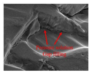
Fig. 2.19 Salt rock pressure dissolution boundary traces (as shown by the red arrow)
