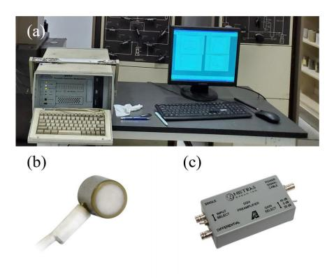
**Fig. 4.2** (a) PCI-2 acoustic emission monitoring system, (b) Nano30 miniature AE sensor, and (c) 0/2/4 type advanced universal voltage preamplifier.
