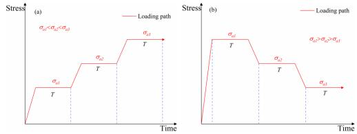
**Fig. 6.4** Loading paths for (a) increasing stress level creep test and (b) decreasing stress level creep test.
