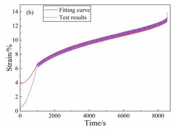
**Fig. 6.9** Comparison graphs of test results and fitting results, (a) with stress upper limit at 90% and stress lower limit at 30%, and (b) with stress upper limit at 95% and stress lower limit at 20%.
