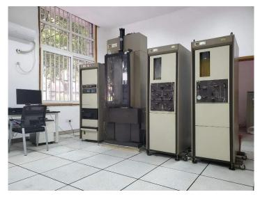
Fig. 2.5 The MTS 815 rock mechanics test system used in this experiment
