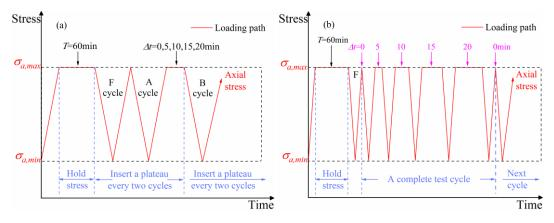
Fig. 2.1 Loading paths for the creep-fatigue tests: (a) CCFs and (b) VCF.
