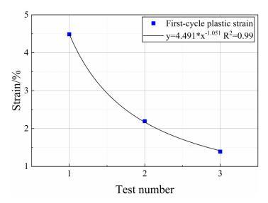
Fig. 5.5 First-cycle strain for three long-time creep-fatigue tests
