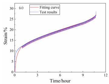
**Fig. 6.12** Comparison graphs of test results and fitting results, (a) uniaxial 5-minute high-stress plateau creep-fatigue test (CCFT), (b) uniaxial 5-minute graded high-stress plateau creep-fatigue (USCF) test, and (c) triaxial creep-fatigue test (TCFT) at a confining pressure of 3 MPa.
