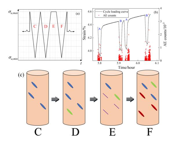
**Fig. 4.17** Typical creep fatigue cycle divided into four stages (a); The strain and AE counts for two cycles in 5th level of USCF test(b); Schematic diagram of salt rock crackles development in typical creep fatigue cycle (c)
