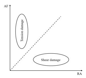
Fig. 4.12 Shear and tensile damage distribution
