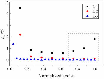
Fig. 5.4 Plastic strain for each complete cycle of the three long-time creep-fatigue tests
