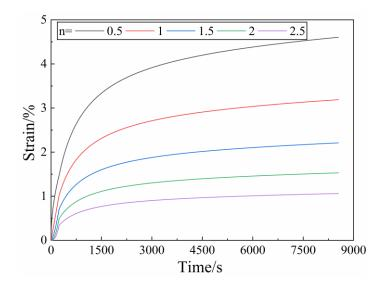
Fig.6.18 Model creep curves under different n values
