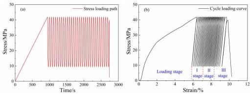
Fig. 6.6 Salt rock fatigue test: (a) stress path and (b) stress-strain curve.
