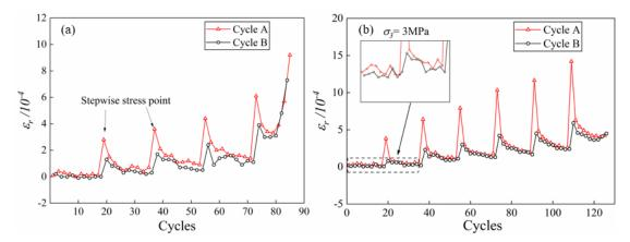
Fig. 4.7 Axial residual strain from each stress cycle during USCF test (a) and TSCF test (b).
