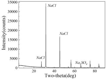
Fig. 2.2 XRD results of the tested salt rock.
