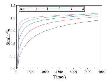
Fig.6.16 Model creep curves under different m values
