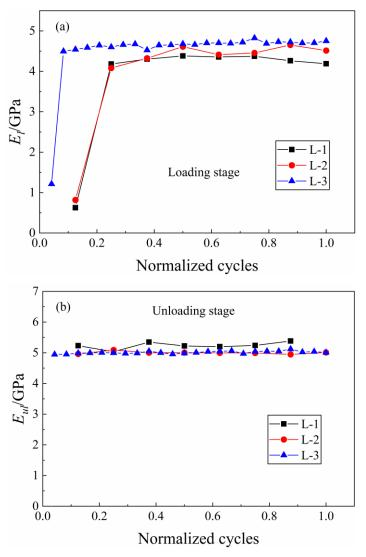
**Fig. 5.7** Elastic moduli computed during (a) loading and (b) unloading for three long-time creep-fatigue tests.
