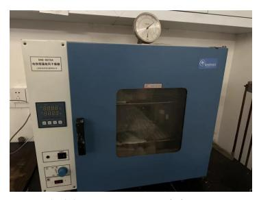
Fig. 2.4 Constant temperature drying oven.
