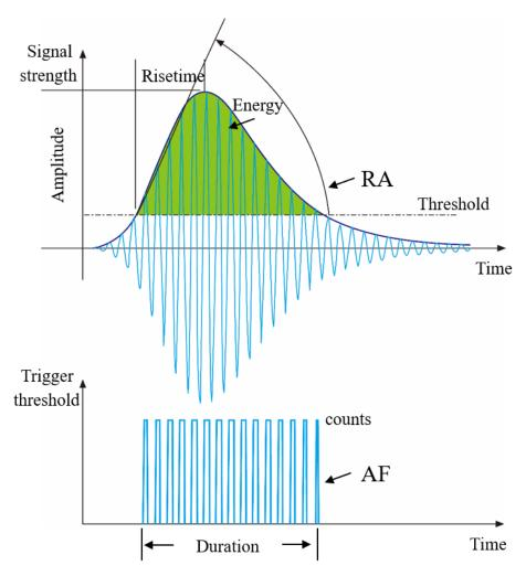
Fig. 4.3 Schematic diagram of typical acoustic emission signal parameters
