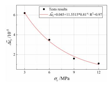
Fig. 3.6 Average residual strain difference between cycles A and B ( $\Delta \bar{\epsilon}_r$ ) for TCF tests under different confining pressure values.
