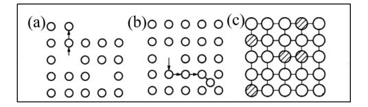
Fig. 2.20 S defect (a), F defect (b) and heterogeneous replacement atom (c).
