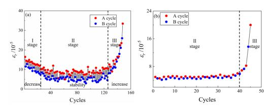
Fig. 3.5 Axial residual strain ( $\varepsilon_r$ ) at each cycle for TCF tests at confining pressure values of (a) 3 MPa and (b) 9 MPa.
