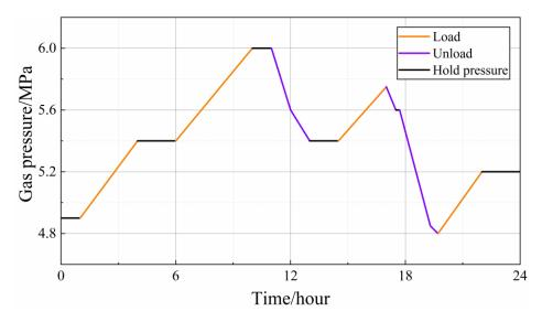
**Fig. 1.8** Schematic diagram of the operating gas pressure of the Huntorf CAES plant within 24 hours.
