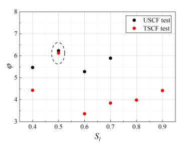
Fig. 4.9 The ratio of creep strain to residual strain  $\varphi$  for every  $S_l$  (excluding the data at the point of abrupt stress elevation) for the USCF test and TSCF test.
