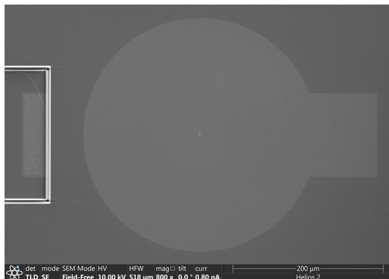
Figure 3.4: SEM view of one of the reference sensor centered on the hole.
