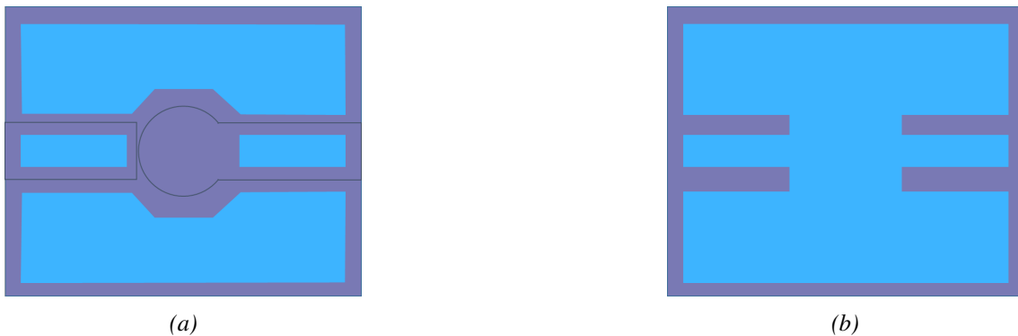
Figure 3.17: Open (a) and short (b) geometries used for de-embedding
