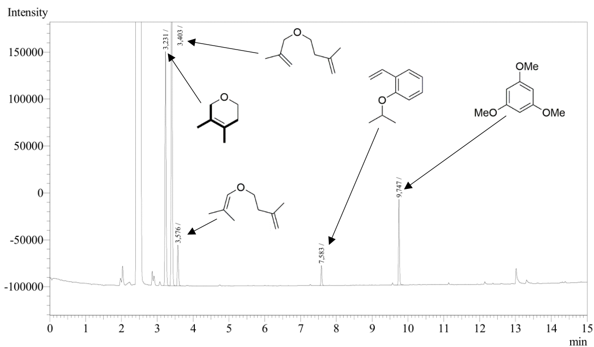
Figure 43 Gas chromatogram of an exemplary reaction mixture from RCM of 84a . Oven temperature program – 100 °C for 5 min.; then 20 °C/min. to 300 °C.
