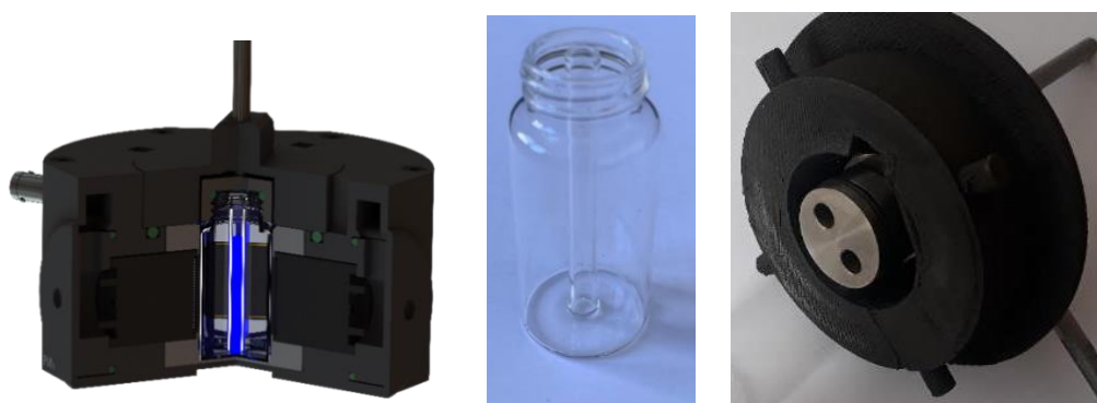
Figure II-15: Showing from left to right - Inside the TDCR device with sample holder; the sample holder; the head of the TDCR device to which the sample vial is screwed and which itself is screwed into the TDCR device.
