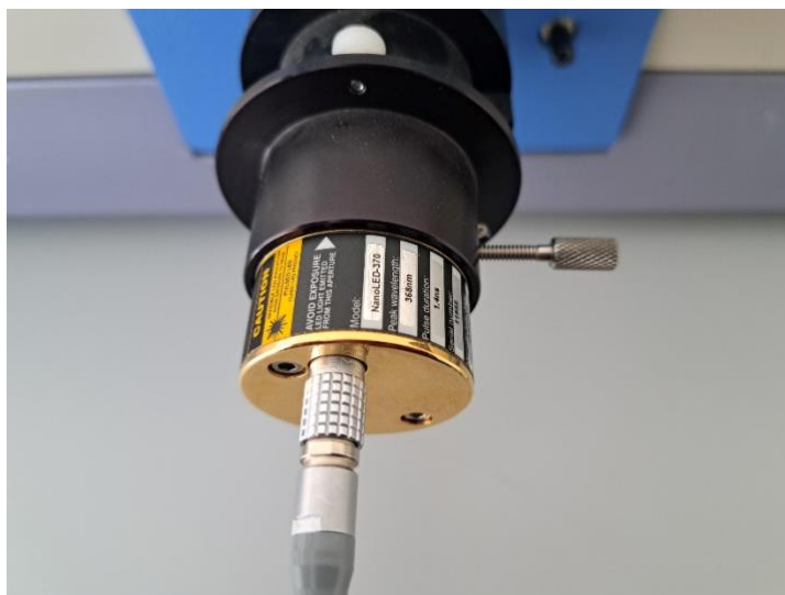
Figure II-9: Showing a pulsed nanoLED connected to the spectrofluorometer.
