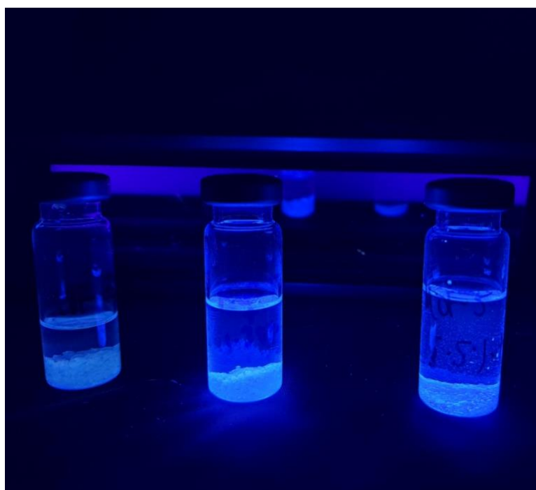
Figure V-12: Showing the fluorescence of a) MOF-5 crystals, b) MOF-5 + 1.38% ADC and c) MOF-5 + 5.5% ADC under an ultraviolet lamp at 365 nm excitation.
