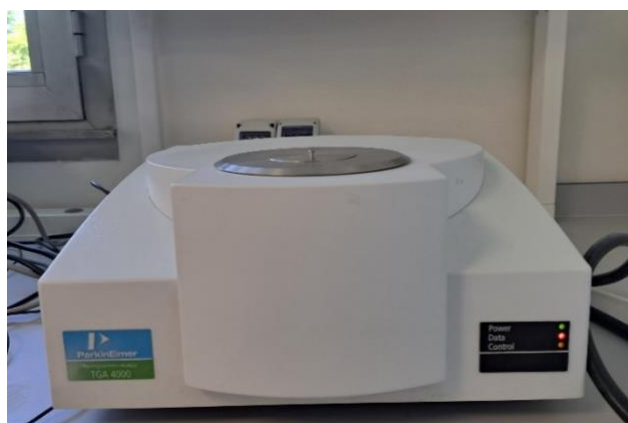
Figure II-4: Showing the TGA setup.
