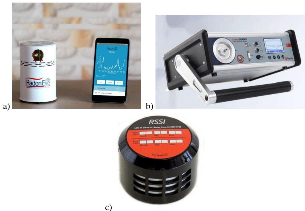
Figure I-5: Illustrating the different commercially available devices for radon detection a) – Radon Eye; b) – Alpha guard; c) – track detector.
