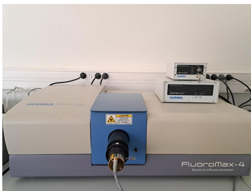
Figure II-7: Showing the spectrofluorometer equipped with a pulsed laser diode (nanoLED) and on the top right the nanoLED synchronous detection devices.
