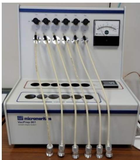
Figure II-2: Illustrating the VacPrep degassing station from Micromeritics.
