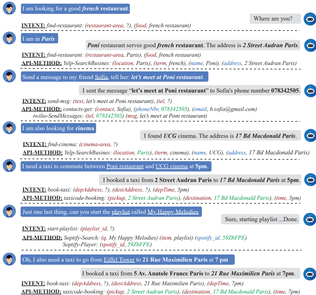
Figure 3.3: Example of multi-turn multi-intent conversation. After each turn, we illustrate the intent, its slot-value pairs, and the API call(s). The red slots/parameters are required input slots/parameters, the blue parameters are output parameters, and the green values are inferred values from different sources.
