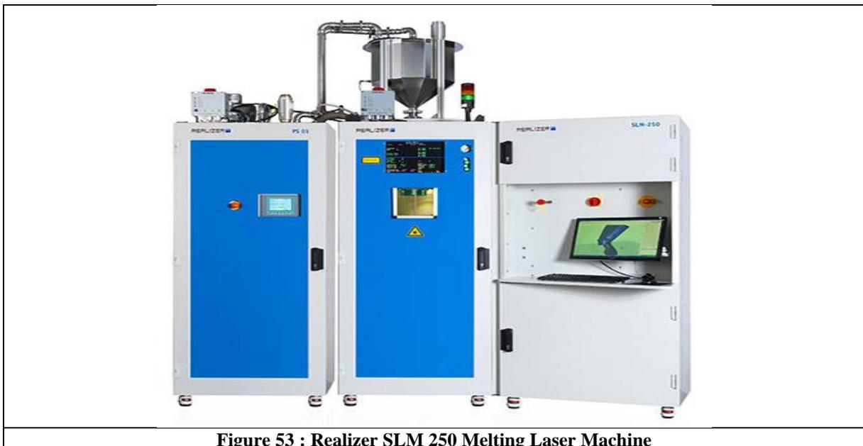
**Figure 53 : Realizer SLM 250 Melting Laser Machine**
