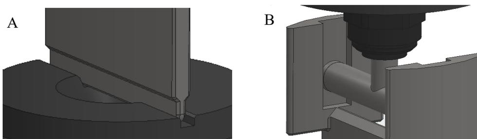
**Figure 38** Support panel (A) and nutrient sparger (B) propped inside the grooves.
