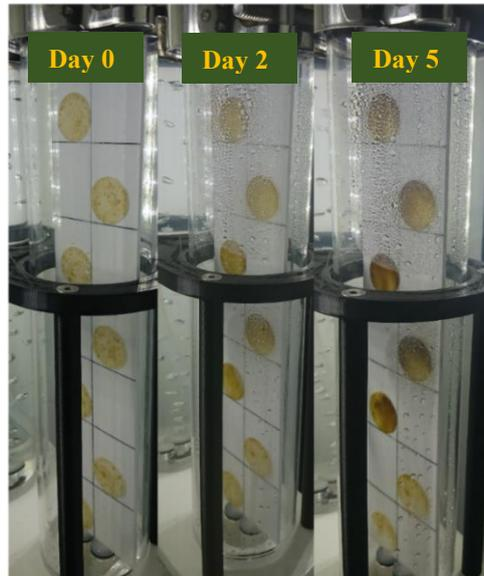
**Figure 29** Progression of *N. laevis* biofilm disks in biofilm PBR following installation (Day 0), Day 2, and Day 5. The biofilms are characterized by variations in color and thickness, which indicate different stages of growth and biofilm maturation.
