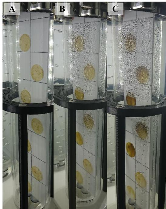
**Figure 20** Growth progression of *N. laevis* in PSBR during (A) launch, (B) day 2, and (C) day 5
