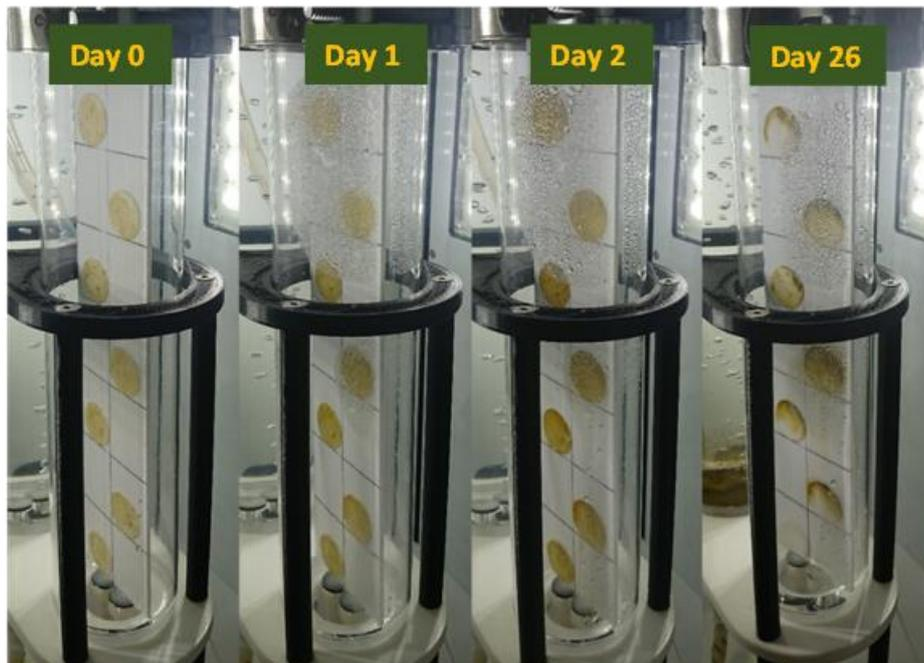
**Figure 31** Progression of *N. laevis* biofilm after 0, 1, 2, and 26 days
