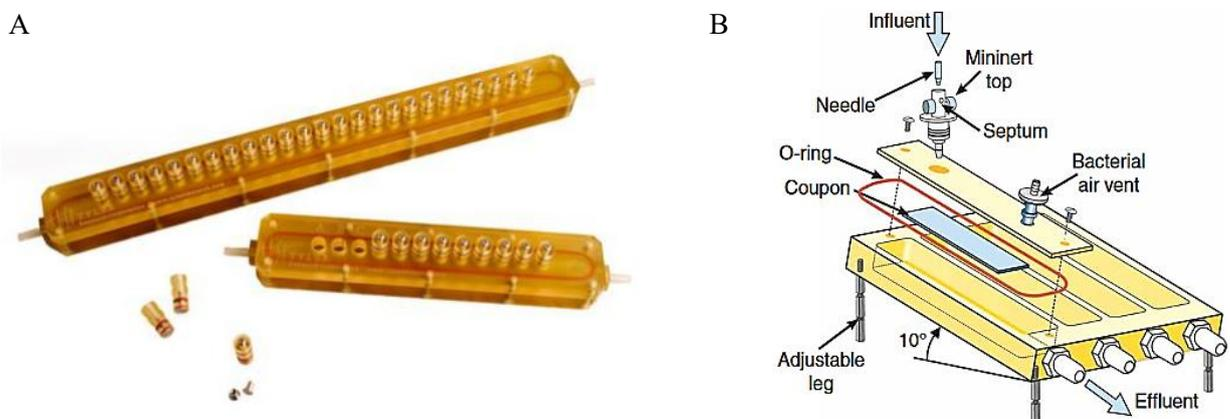
**Figure 16** Flow chamber systems used to investigate biofilm development. A) Multiple ports in a closed Low Pressure Modified Robbins Device (LPMR) setup allow for simultaneous biofilm screenings (© Tyler Research Corporation). B) The Drip Flow Biofilm Reactor (DFR) has a tilt angle of  $10^\circ$  and a designated outflow port to drain planktonic cells, allowing true biofilm cells to be retained on the coupon (Mannix-Fisher, 2021).
