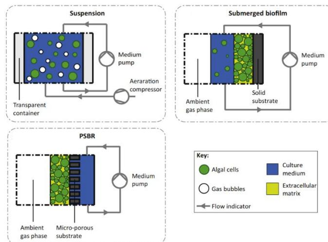
**Figure 23** Schematic representation of three different bioreactor configurations for the cultivation of algal cells: a suspension-based system, a submerged biofilm system, and a PSBR (Podola et al., 2017)
