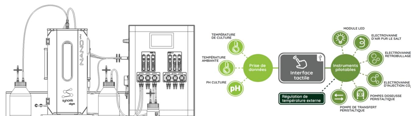
**Figure 24** Functional scheme of NANO photobioreactor
