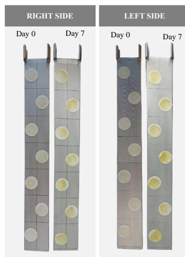
**Figure 45** Photographic comparison of biofilm disks inoculated on the left side and right side of the PSBR support panel on the day of launch (Day 0) and after harvest (Day 7).
