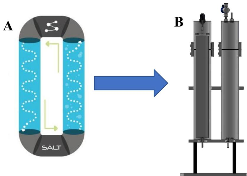
**Figure 25** Schematic overview illustrating the transformation of Synoxis' NANO culture chamber from a suspension-based technology (A) to a biofilm-based system (B), highlighting the adaptation of the technology for different methods of algal cultivation.
