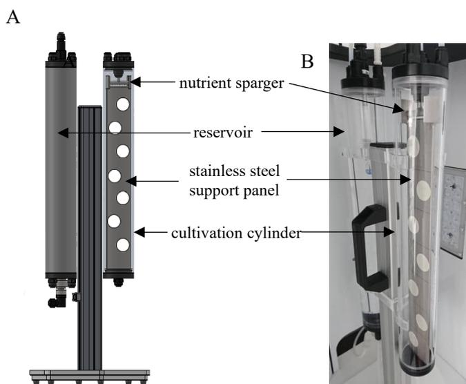
**Figure 39** PSBR setup, adapted from an existing PBR for suspension cultivation, and currently composed of the cultivation (left) with steel panel covered by a lens tissue and supporting filters inoculated by diatoms; and the reservoir (right) cylinders (A)
