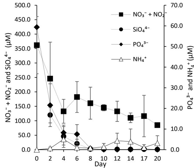
**Figure 44** Average nutrient availability ( $\text{NO}_3^- + \text{NO}_2^-$ ,  $\text{PO}_4^{3-}$ ,  $\text{SiO}_4^{4-}$ , and  $\text{NH}_4^+$ ) in Fernbach flasks culture media at every sampling interval (except for  $\text{SiO}_4^{4-}$  without day 0). Error bars represent standard deviation ( $n = 3$ ).
