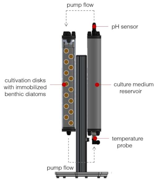
**Figure 21** Schematic diagram of improved Synoxis Algae PSBR
