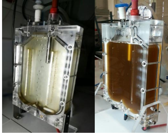
Figure 19 Growth of marine benthic diatom (A) Amphora sp. NCC169 and (B) Entomoneis paludosa in an airlift photobioreactor (©Eva Cointet)
