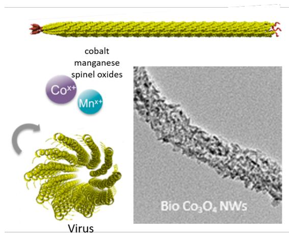
Figure 1.7: **Colloidal nanowires.** Filamentous virus capped with cobalt manganese spinel oxides on their surface function as templates for the fabrication of battery electrodes. [40]
