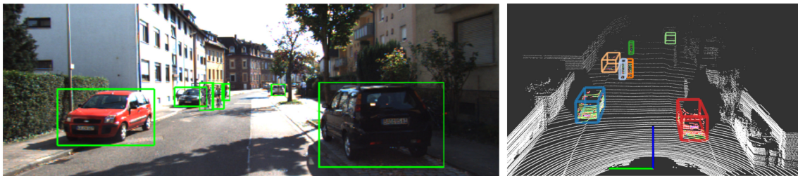
Figure 4.1: Schematic diagram of 2D detection in images and corresponding 3D detection in point clouds.
