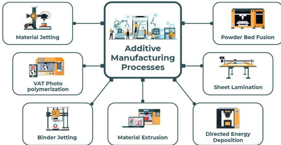
Figure 7: The seven existing 3D printing processes
