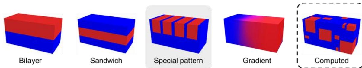
*Figure 49: Multi-material distribution categories. The special pattern is considered in this study to further master the fabrication of computed materials distributions.*
