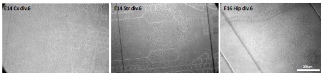
Figure 92. Three neuronal subtypes (Cx : cortical, Str : Striatal, Hip : Hippocampal) seeded in a two nodes network chips fabricated by route A co-patterning techniques. Note that adhesions “contrast” is poor with many cells growing on PEG-PLL areas.
