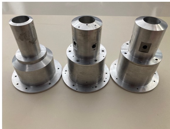
Fig. 2.1 Subscale DBN models: Smooth, injection 8 mm, and injection 16 mm (from left to right)
