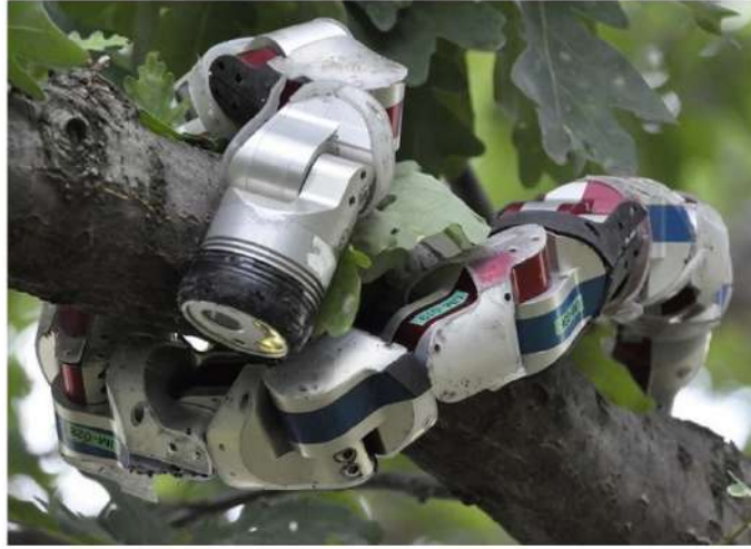
Figure 1.1: An hyper-redundant manipulator working in a confined environment, courtesy of [4].
