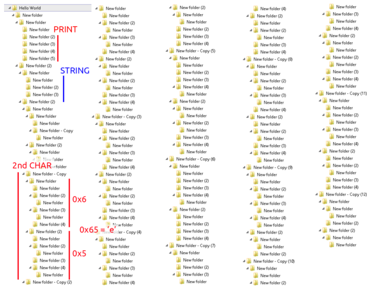
Figure 5.1: Implementation of the traditional "Hello, world!" program in the Folders programming language. (Temkin, 2015)
