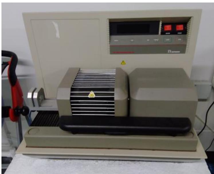
Figure 89 ATG TA instrument Q100
