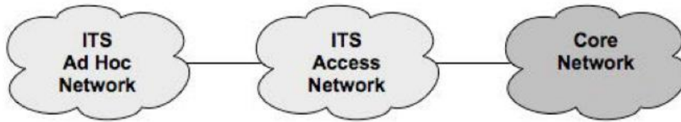
Figure 9. High-level ITS network architecture: Ad hoc-centric
