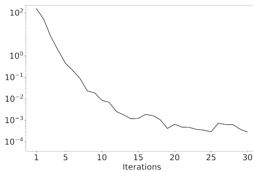
Figure 5.4: Evolution of the MSE w/LU at Dirichlet nodes across the different iterations of an inference.
