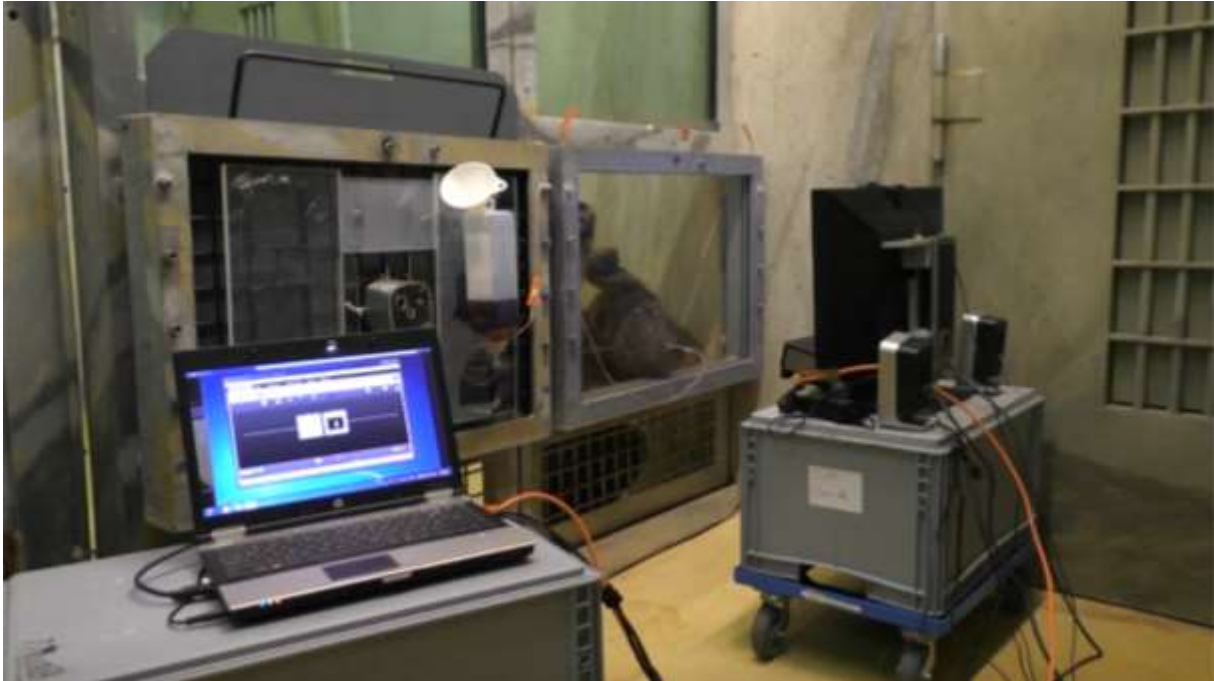
Figure 2 : Eye-tracking setup used by Krupenye et al. [88]. An infrared eye-tracker non-invasively records an orangutan's gaze as she attends to pictures and videos presented on a monitor, just outside of her enclosure. A nearby laptop controls stimuli presentation. Subjects voluntarily approach the setup to view the stimuli and sip a slow stream of juice. Copyright: Christopher Krupenye and Leipzig Zoo. From Krupenye et al (2019) [83]. Reproduced with consent.
