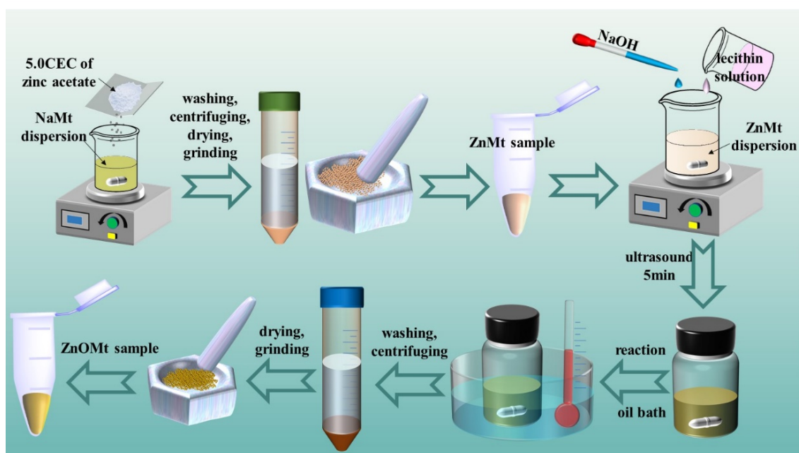
Fig. 6.1 The schematic representation of experimental workflow for preparing ZnOMt samples
