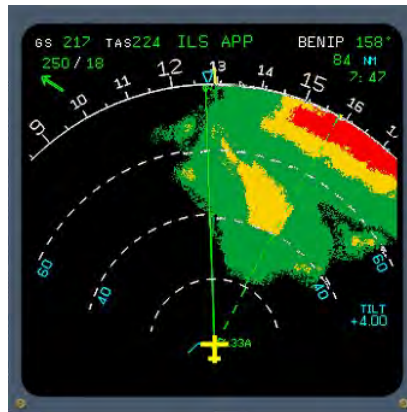
Figure 3.2: Meteo Radar information display. The colored areas correspond to cloudy areas. Those in green do not pose a safety problem. On the other hand, those in red have to be avoided.
