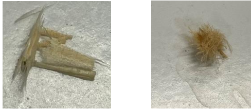
Figure 18: Strands of spruce taken from CLT (left), and loose fibers taken from wood fiber board (right)
