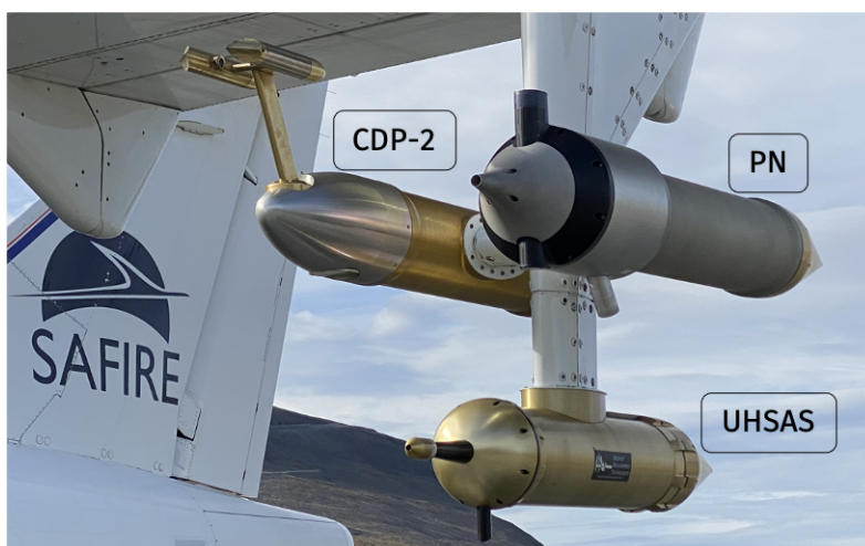
Figure 2.6: The Polar Nephelometer on the ATR 42 scientific aircraft during the RALI-THINICE campaign.
