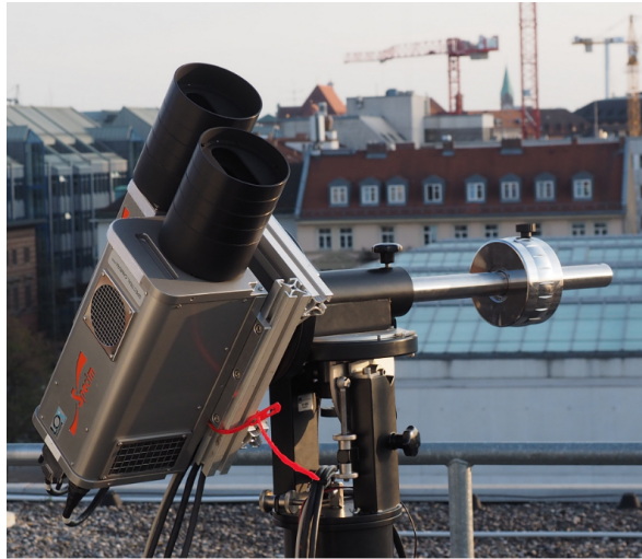
Figure 2.14: The specMACS VNIR and SWIR cameras, ground-based on the roof of the Meteorological Institute in Munich and protected from stray light by black protection visible in the front on the sensors (from Ewald et al. 2016).
