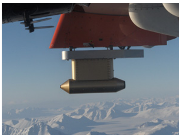
Figure 2.1: The Cloud Particle Imager on the Dornier 228 Polar 2 aircraft flying over the Svalbard archipelago. (from C. Gourbeyre, http://www.obs.univ-bpclermont.fr/atmos/fr/recherches/campagnes/astar2007.php )
