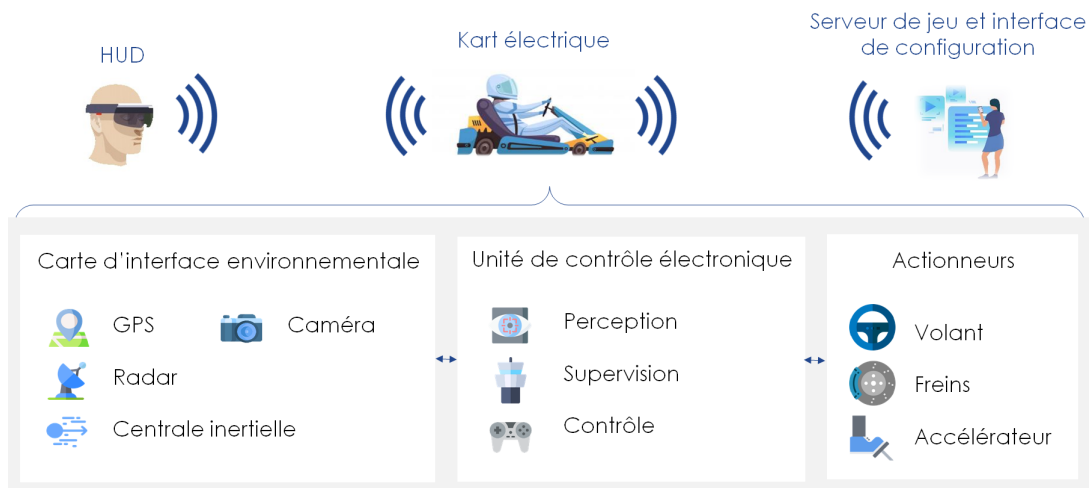
FIGURE 1.3 – Diagram summarizing the communications between the entities of the KARlab project, as well as the modules present on board the kart
