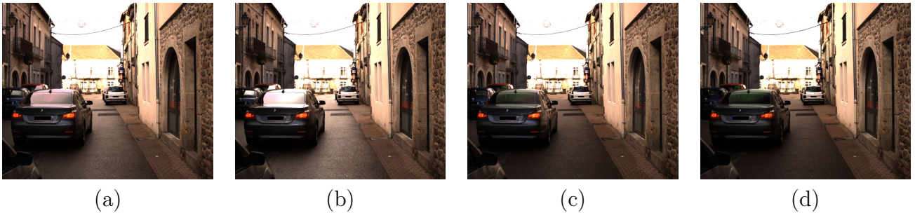
Figure B.8: Specularity removal application results. (a) Unfiltered, total intensity. (b) (c) Filtered image by simulating a linear polarization filter oriented at 60^\circ , and 120^\circ , respectively. (d) Polarized specularity removal by filtering with the Degree of Linear Polarization.
