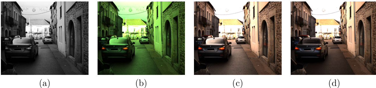
Figure B.4: (a) Raw, mosaiced version of the reference image, for the polarization channel 0^\circ . (b) Demosaiced version of the reference image, without white-balance, for the 0^\circ polarization channel. (c) White-balanced, demosaiced images for the polarization channel 0^\circ . (d) White-balanced, demosaiced images for the polarization channel 135^\circ .
