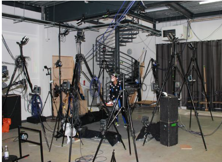
Figure 1.2: MocapLab’s motion capture system and field for sign language motion acquisition.
