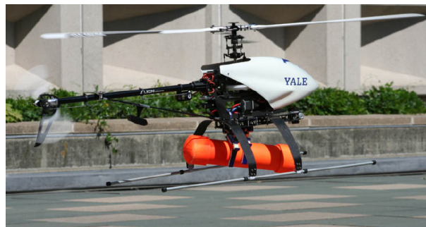
Figure 1.2 – Yale aerial manipulator test-bed with mounted gripper [11].
