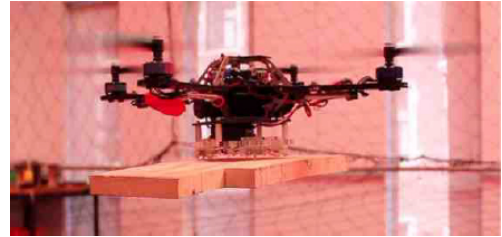
(b) The flat piece of wood is held by an ingressive gripper.
