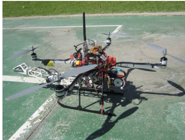
Figure 1.8 – Quadrotor with 3-DOF manipulator arm developed by [17].
