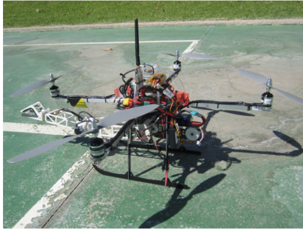
Figure 1.8 – Quadrotor with 3-DOF manipulator arm developed by [17].
