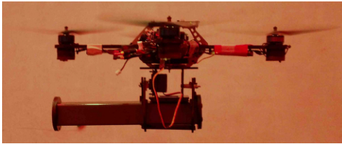
(a) The beam is grasped with an impactive gripper.
