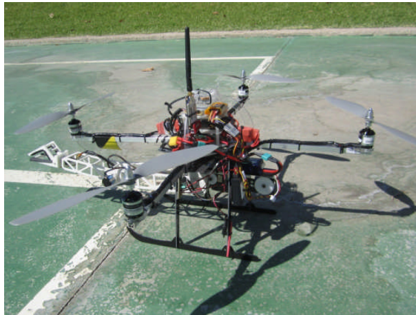
Figure 1.8 – Quadrotor with 3-DOF manipulator arm developed by [17].
