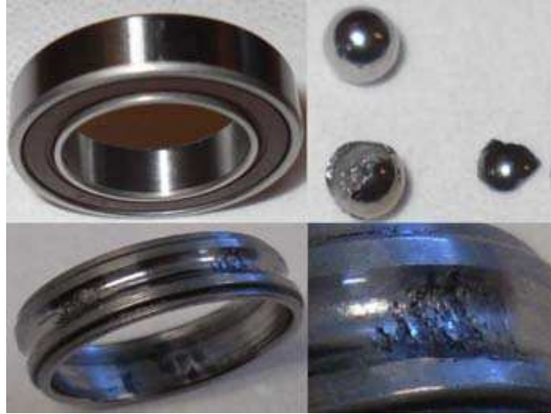
Figure IV.12: Image of bearings issued from the experimental platform of [135] and their degradations
