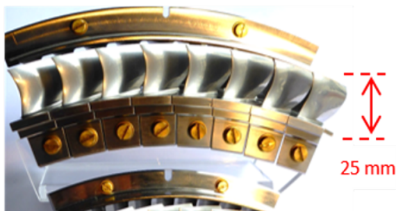
Figure 4.1. H25 compressor blades
