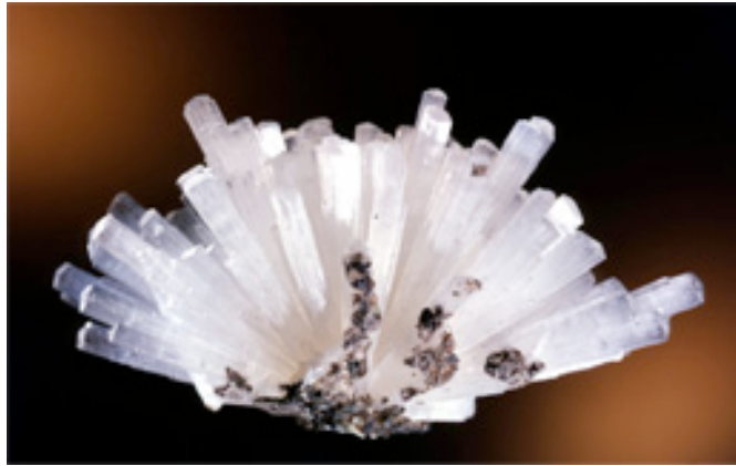
Figure 1.1 Natrolite (Image from the Commission on Natural Zeolites and courtesy of Olaf Medenbach).
