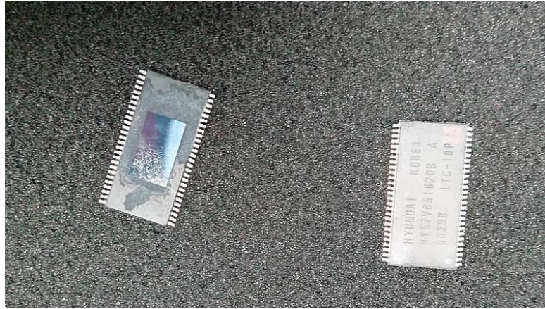
Figure 95: DRAM delidded backside (left) and front side (right).
