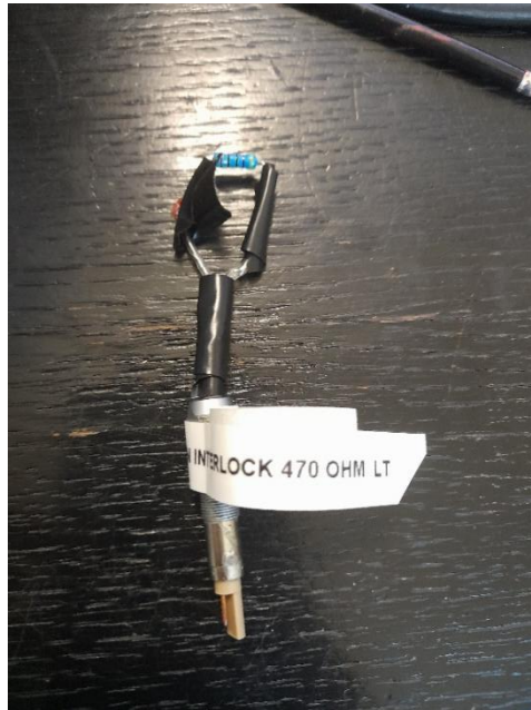
Fig. 51: The gyrotron is interlocked with the resistor connected to it.
