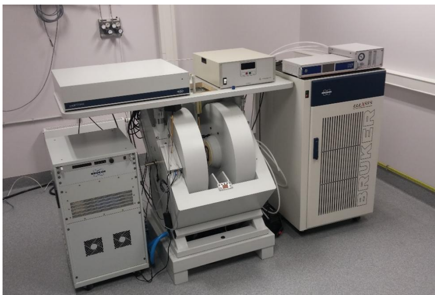
Fig. 11: BRUKER EPR Spectrometer with the microwave bridge, magnet, and electronics console.
