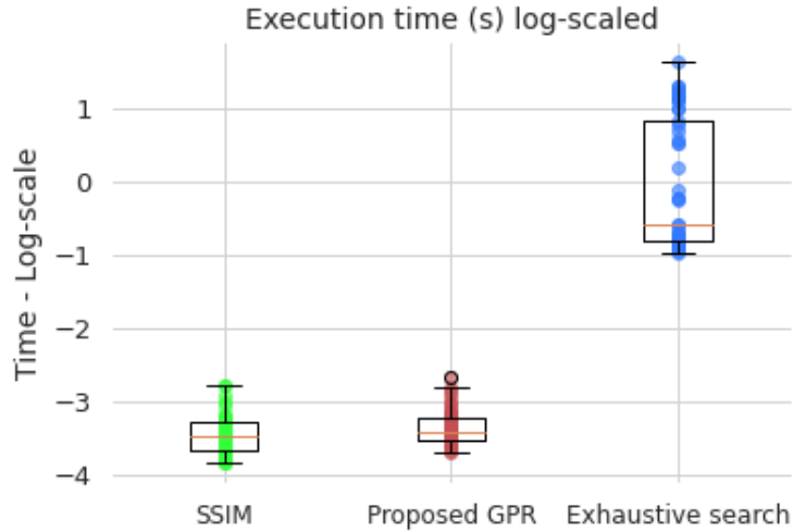
Figure 5.4: Boxplots of execution times of our proposed approach, of the SSIM and the exhaustive search method on 3D dose distributions. Our implementation of the gamma index is faster than the open-source exhaustive search method. Its speed is comparable to the execution time of the SSIM, thus ensuring tractable trainings of deep learning models.
