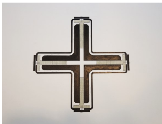
Figure 106 : Détail du dessin German Pavilion, International Exposition, Barcelona, Spain Horizontal column section , Ludwig Mies van der Rohe, 1929, inv.°1000.196. ©M.Cinquabre/The Museum of Modern Art, New York/VG Bild-Kunst, Bonn
