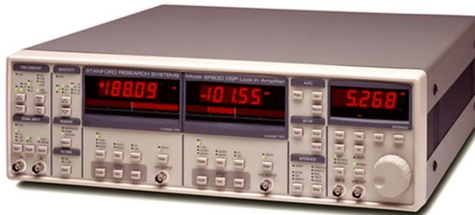
FIGURE A.5 – Model SR 830 DSP Lock-in Amplifier.
