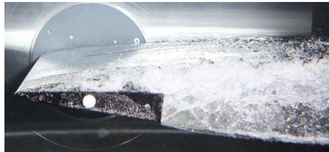
FIGURE I.23 – Supercavitation autour d'un hydrofoil (Pearce et Brandner [184])
