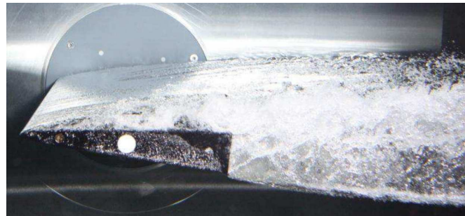
FIGURE I.23 – Supercavitation autour d'un hydrofoil (Pearce et Brandner [184])
