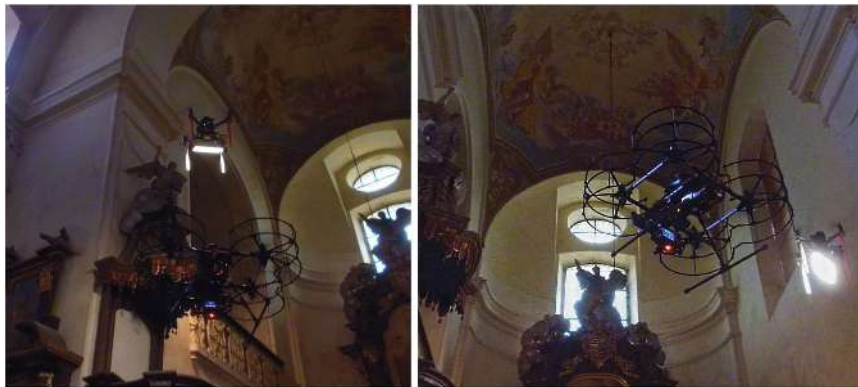
Figure 1.19: UAV based RTI acquisition introduced by Krátký et al. [2020]
