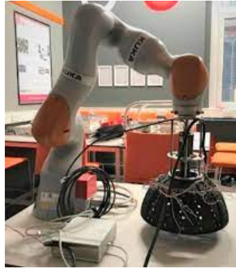
Figure 1.18: Acquisition system by Chen et al. [2020] based on robotic arm and fixed dome for large-scale 3D surface imaging.
