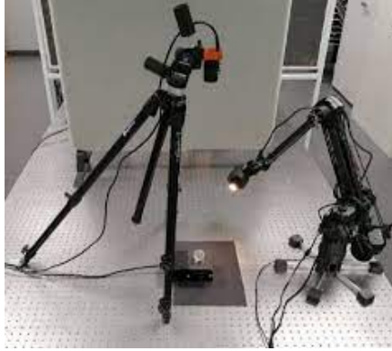
Figure 1.20: Robotic arm based RTI acquisition set up by Kitanovski and Hardeberg [2021]
