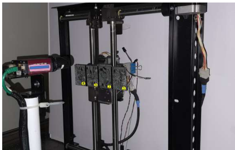
Figure 2.20: An example of batch acquisition where the system executes acquisition of 4 surfaces one after the other.
