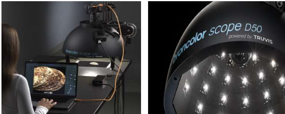
Figure 1.16: An example of fixed light dome RTI acquisition system. This system is a model Scope D50 system from Broncolor Swiss, containing 50 evenly spaced LED lights. Images from bro
