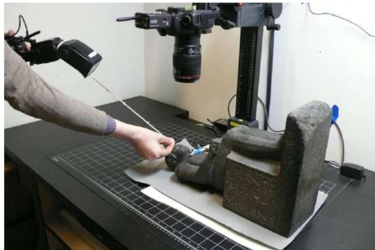
Figure 1.15: Highlight-RTI being performed with handheld light source and camera held by a mechanical support. Picture courtesy: NCPTT
