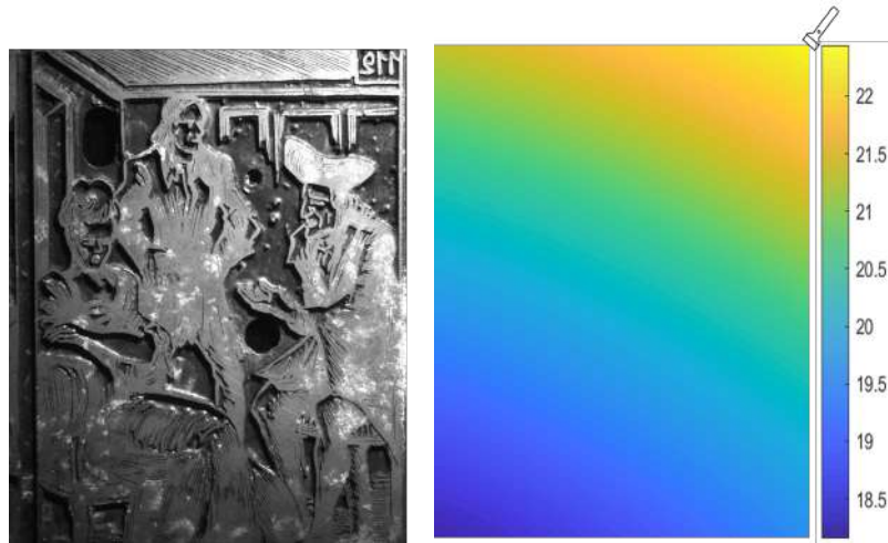
(b) Illumination across the surface. The left image shows the captured image of the illuminated surface, the right image illustrates the variation in energy distribution on the surface points through a heat map representation, with brighter areas indicating higher levels of energy and darker areas indicating lower levels.
