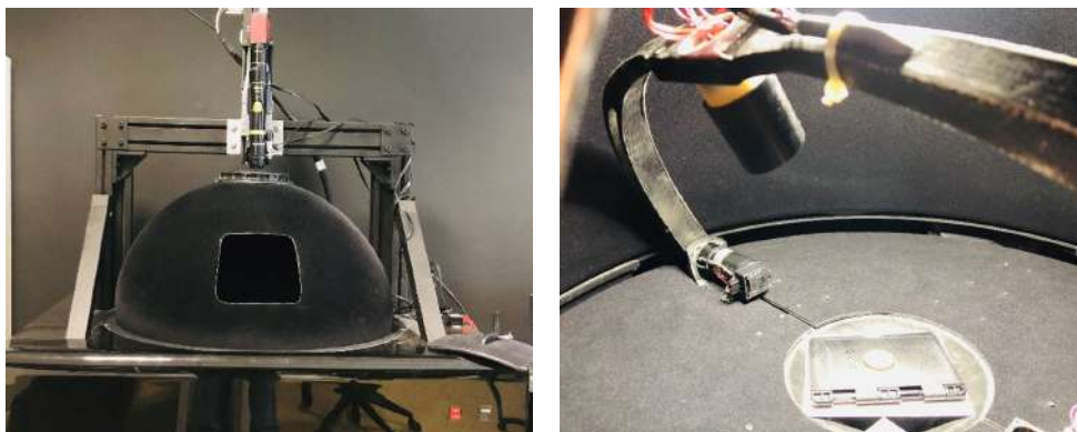
Figure 1.17: An example of mechanized dome RTI acquisition system. In the image on the right, we can see a light source attached at the apex of a semi circular rig, that eventually is attached to a motor and a rotating disc. This system is built inhouse in Imvia Laboratory (Universite Bourgogne, Dijon, France).
