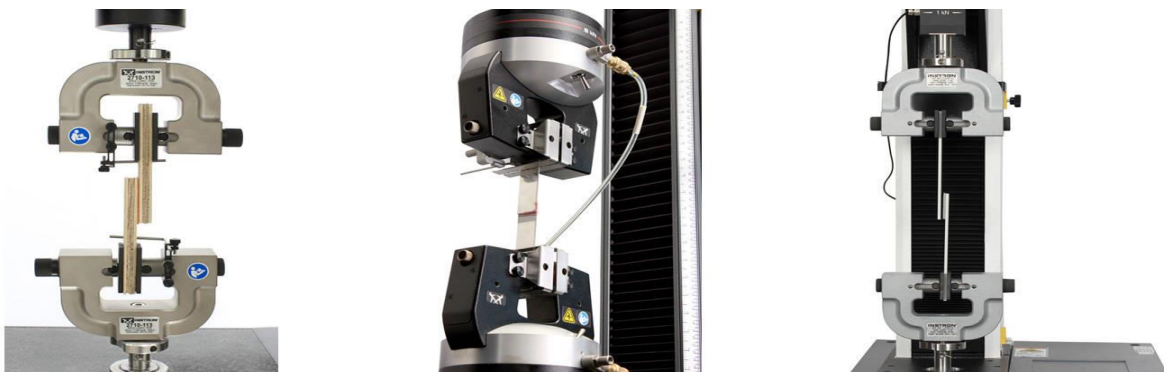
Figure I.10: Tensile test used to measure the adhesive shear bond strength of rigid-to-rigid assemblies [130]
