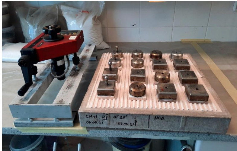
Figure I.7: Samples prepared for the pull-off test [128]
