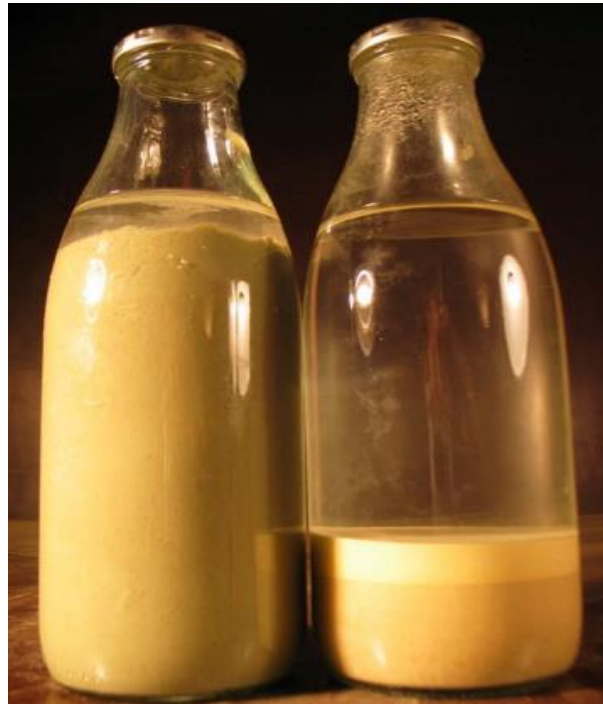
Figure II.11: Difference in Water Swelling Between Kaolinite (Right) and Smectite-Type Swelling Clay (Left) [185].
