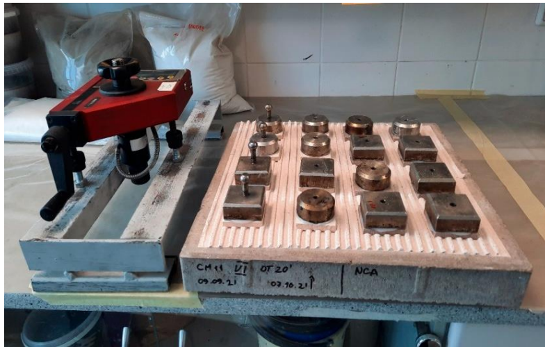
Figure I.7: Samples prepared for the pull-off test [128]
