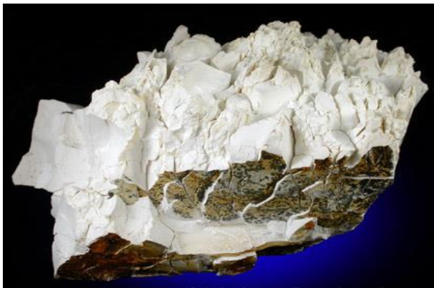
Figure II.9: White mass of Kaolinite with many shrinkage cracks. Several faces are covered with dendritic patterns of manganese oxide. Ex. A. Lincoln Sherk II, MD. (1896-1970) [183]
