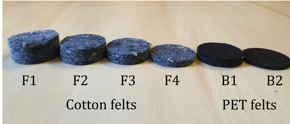
FIGURE III.1 – Felt samples thermobonded at different thicknesses (sample diameter, 45\text{mm} ).
