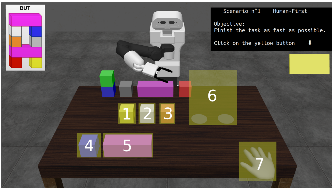
Figure 5.4: Hidden clickable areas triggering human actions, if feasible. Areas from 1 to 5 trigger picking the respective cube if it is on the table and the human is not holding one already. Area 6 corresponds to placing a held cube in the stack. Area 7 makes a hand gesture indicating the human desire to be passive to the robot.
