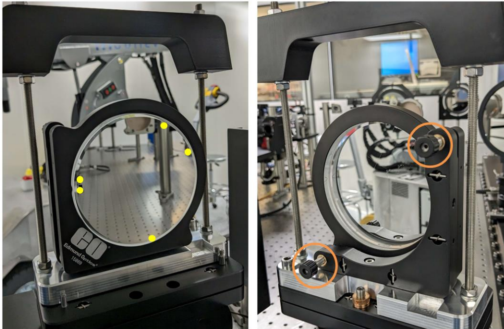
Figure 68: Dummy mirror mounted in its holder. (Left) Front face, with five markers (yellow). (Right) Rear face, with holder adjustment screws circled in orange.
