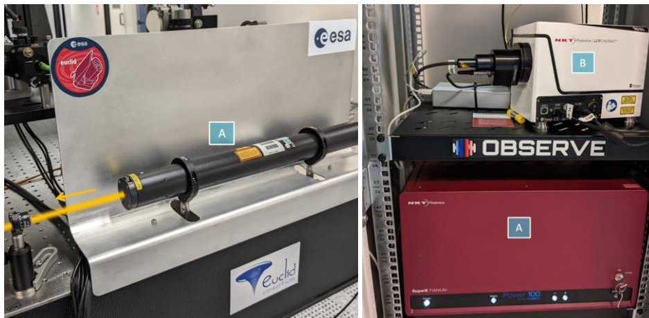
Figure 44: (Left) Reference source. (Right) Polychromatic source and monochromator.
