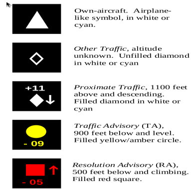
Figure 4.2: Standardized Symbology for Use on the Traffic Display
