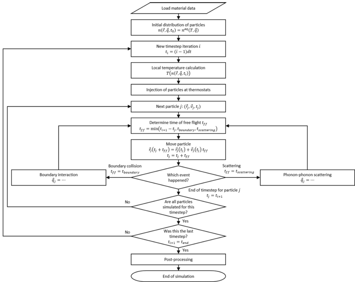
Figure 2.5 Flowchart of the Monte Carlo algorithm for phonon transport simulation, adapted from [259].
