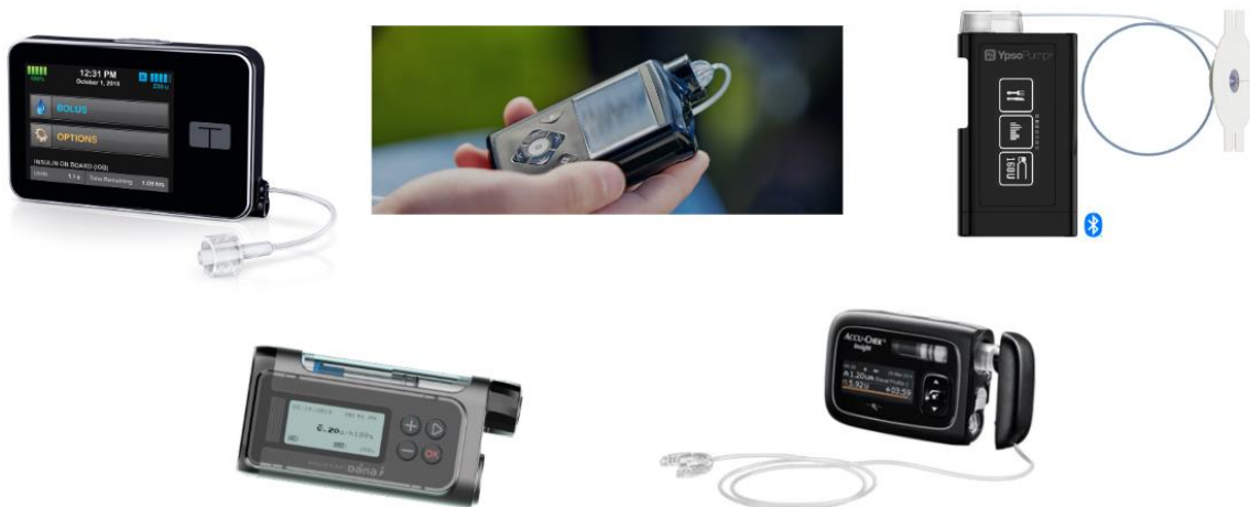
Figure 1 : A few examples of insulin pumps (from left to right and from top to bottom: a t:slim x2 (Tandem), a Medtronic 780G (Medtronic), an Ypsopump (Ypsomed), a Dana i (Dana), and an Accu-Chek Insight (Roche Diabetes)).
